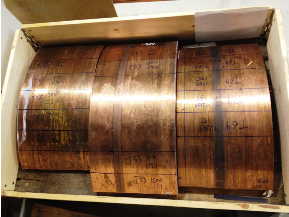
Figure 1. The three different tube parts received for testing. The markings show the different positions for the creep specimen blanks.
