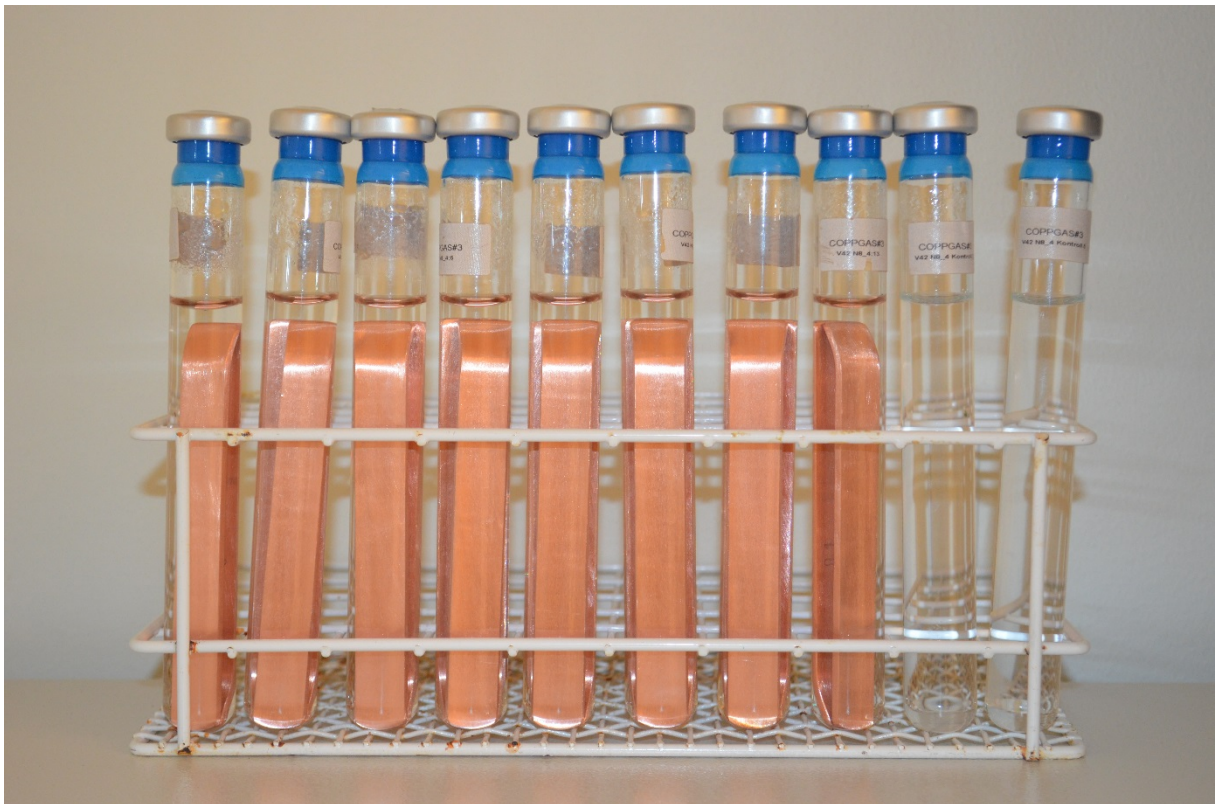
Figure 4-15. Image of N8 vials after 806 days. Vials N8:1, 2, 3, 5, 8, 9, 11, 13 are shown from left to right plus two vials with water only.
