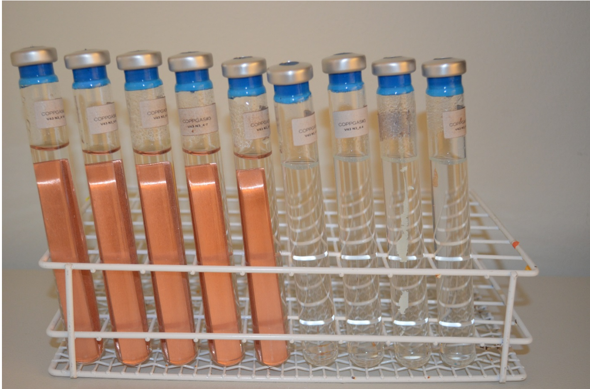
Figure 4-12. Image of N3 vials after 846 days. N3:6 to N3:10 with copper and water and N3:2 to N3:5 with water only are shown from left to right.
