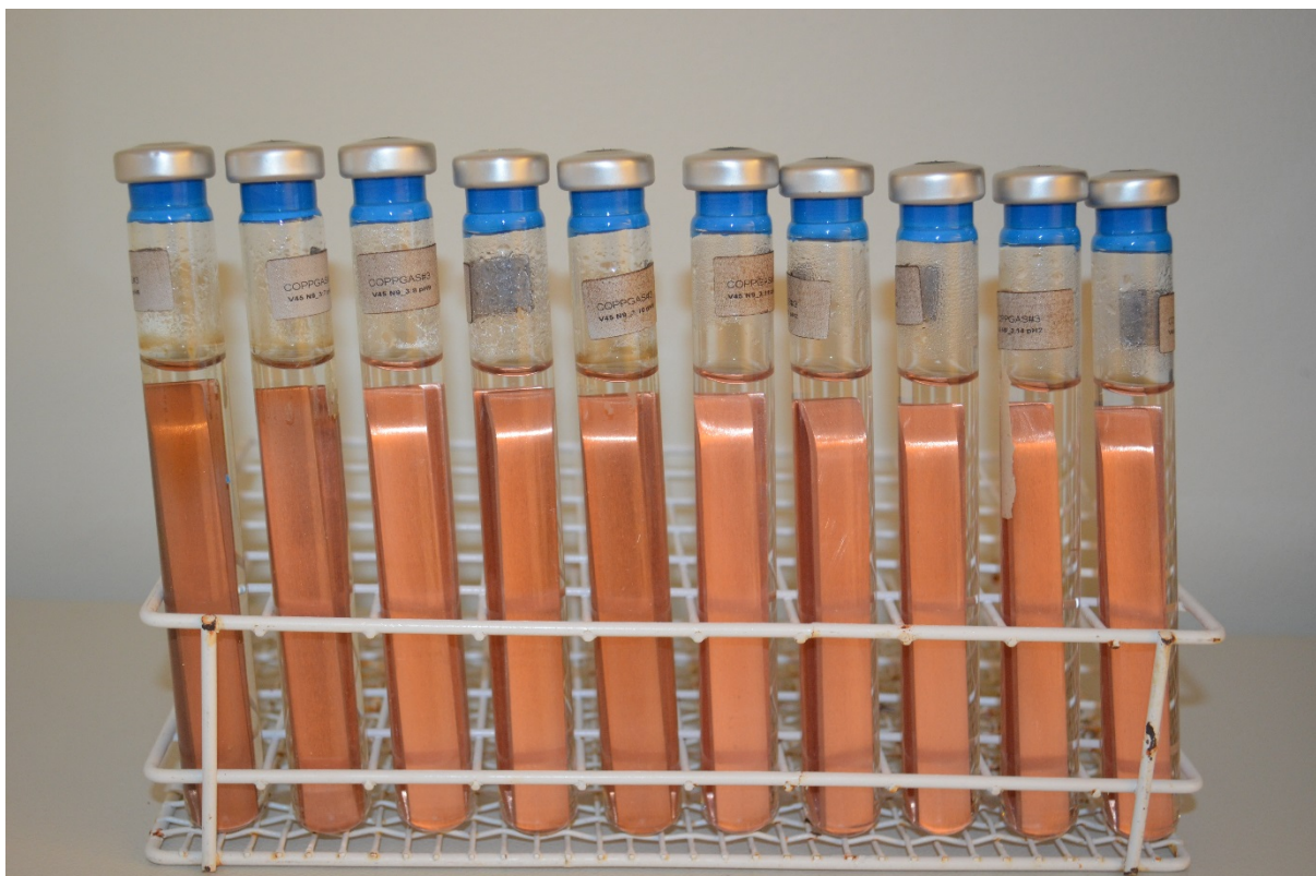
Figure 4-16. Image of N9 vials after 788 days. N9:6 to N9:15 are shown from left to right.
