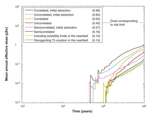
Figure 2. Summary of far-field mean annual effective dose for probabilistic calculations for the corrosion scenario. The peak doses are given in parentheses in  $\mu$ Sv.
