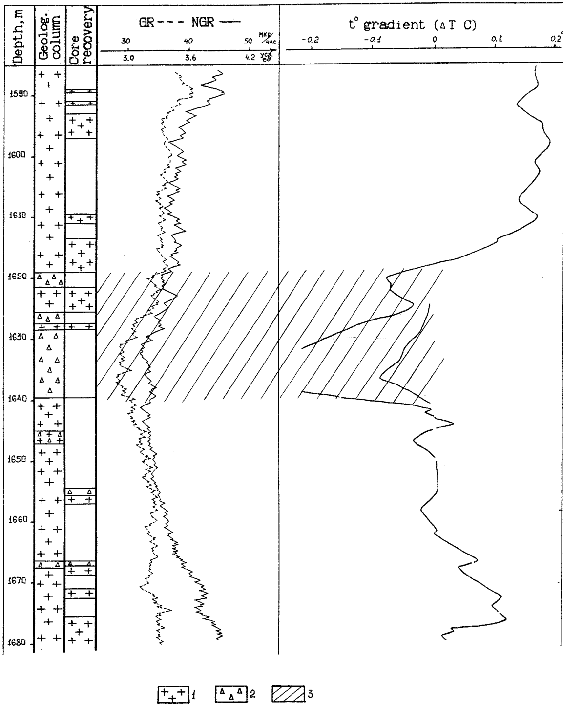
Fig. 5-9. Characteristics of a fracture zone in the interval between 1620 and 1647 m in the Tyrnauz borehole
