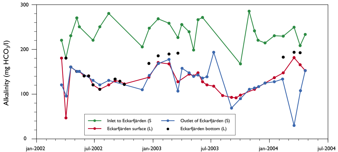
Figure 4-50. The alkalinity in Lake Eckarfjärden (L) and its inlet and outlet streams (S). The observations in the lake are separated according to sampling depth.
