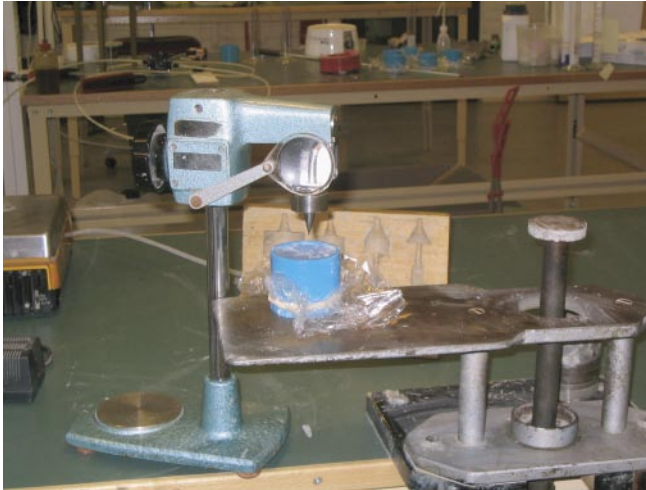
Figure 4-9. Fall-cone apparatus. The blue cylinder contains silica sol for shear strength test. /Axelsson, 2004/.
