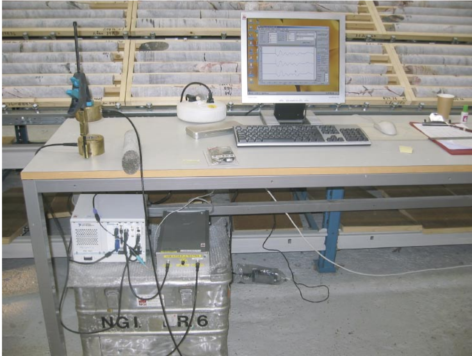
Figure 3-2. NGI's equipment set-up for measuring acoustic P-wave travel time transverse a foliated borehole core.
