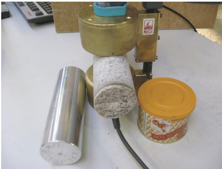
Figure 3-1. Detail of NGI's apparatus for measuring acoustic P-wave travel time transverse a foliated borehole core. The aluminium cylinder for calibration of the device is on the left.
