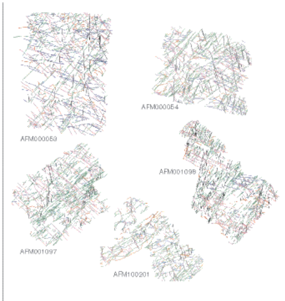
Figure 5-66. Fracture trace maps with the different sets identified in outcrop shown with different colours. North is directed upwards in the figure. The different trace maps are at different scales (see also Figure 5-31).
