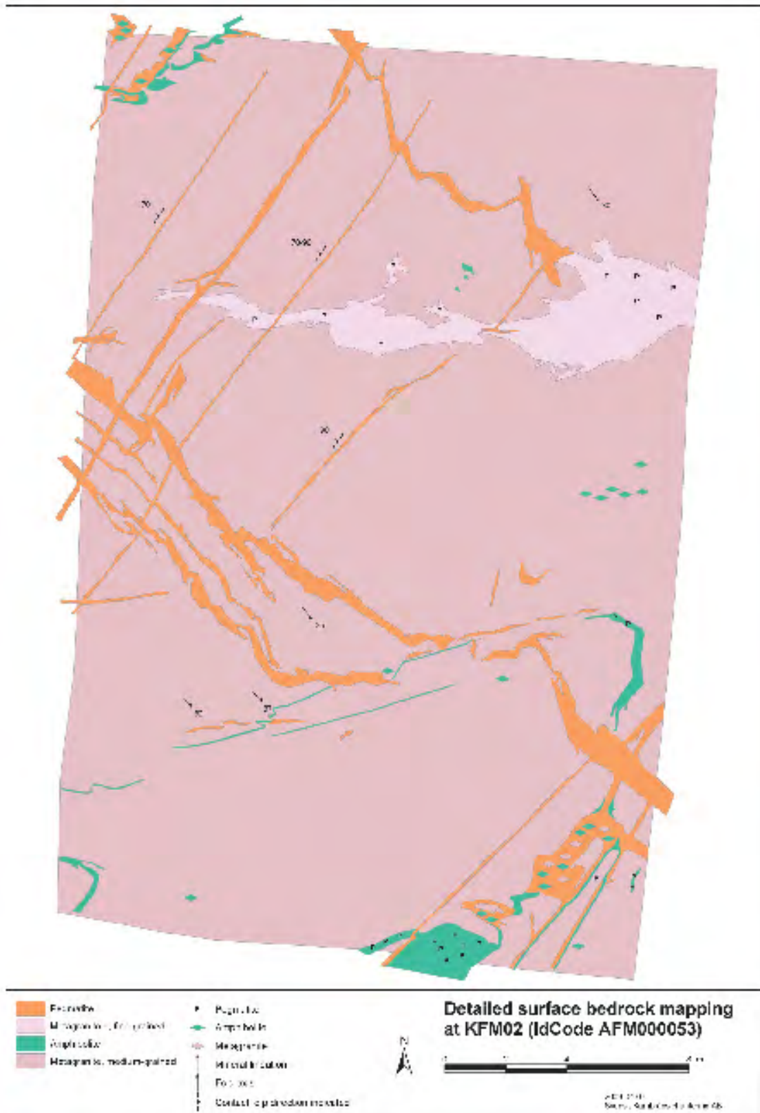
Figure 5-15. Detailed geological map of drill site 2 (after Andersson and Bergman in /Hermanson et al. 2003a/). With the exception of some faults, all fractures in the bedrock have been omitted from the map for purposes of clarity.
