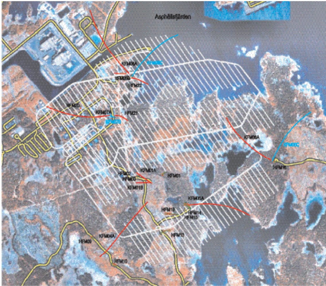
Figure 3. Possible repository layout at 400 m depth in the prioritised area /layout version from Ramböll to SKB, February 2005/. This design is based on the results of SDM, version 1.2. Boreholes (including KFM06C, KFM07B and KFM08C) are also shown with known or predicted orientation diversions.
