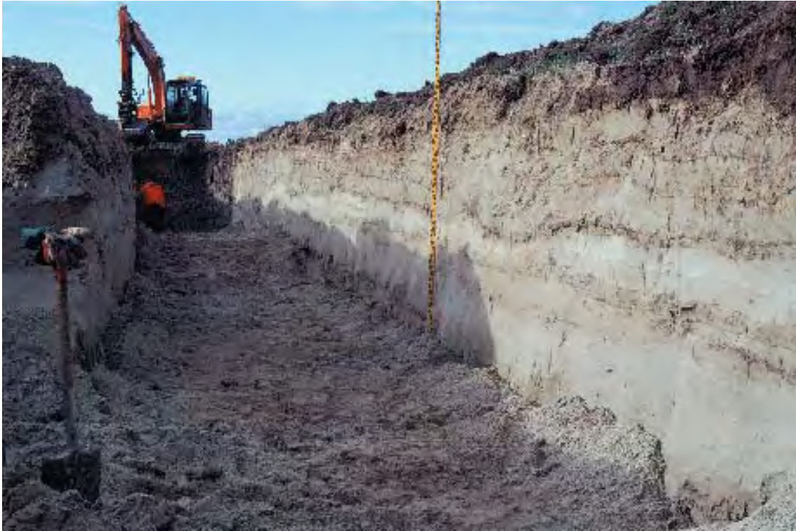
Figure 3-7. This section is typical of the stratigraphy along the Börstil esker. The trench section shows a bed of fine sand and coarse silt covered by a bed of clay-laminated silt. Extended excavation revealed loosely packed and saturated glaciofluvial sand to a depth of at least 5 m. Although the stratigraphy is considered to be highly susceptible to liquefaction, no disturbances related to seismically induced liquefaction were discovered here or elsewhere along the Börstil esker.
