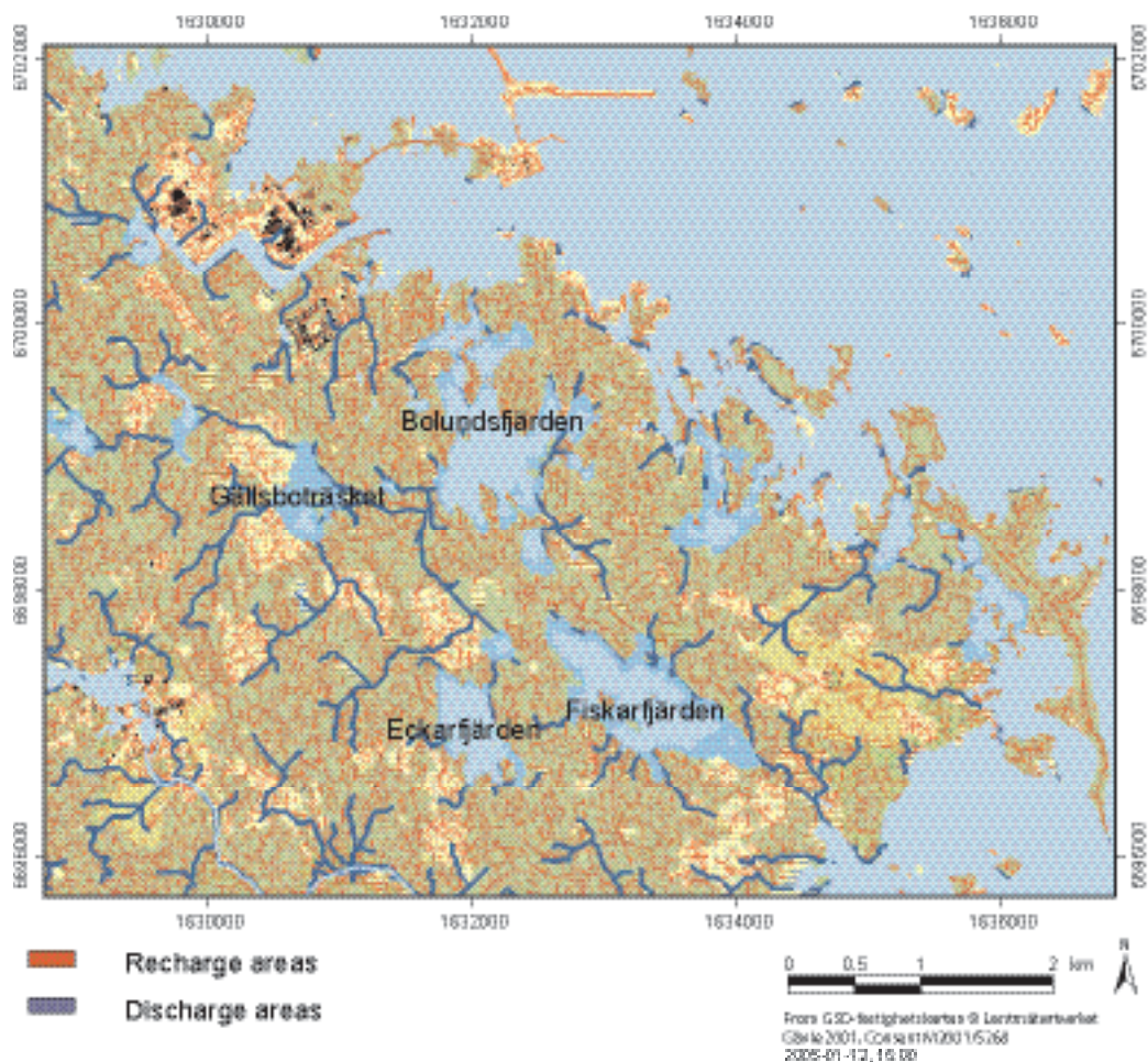
Figure 4-7. Identification of recharge and discharge areas using a GIS model. Areas with colours other than blue and red are “intermediate areas”, i.e. neither recharge nor discharge areas based on the definitions of those in the modelling (see text).
