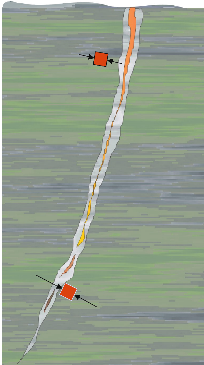
Figure 5-30. Schematic view of a fracture zone, its core and the zone of influence, tapering off towards the deep end. Because of the lower portion being stiffer, the fracture zone is less prone to shearing over that section.
