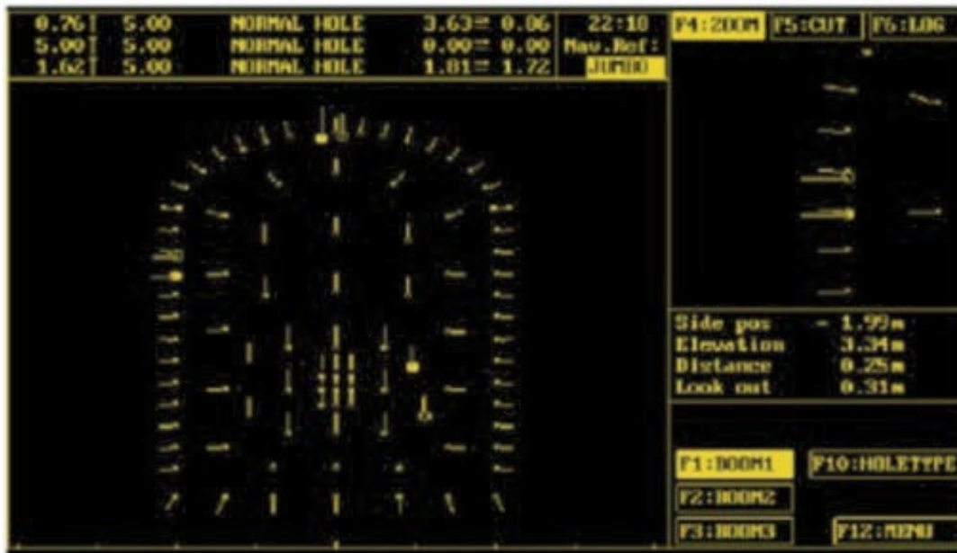
Figure 6-11. The drill plan as displayed for the operator.
