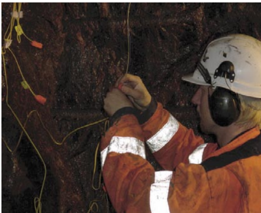
Figure 6-17. Connecting the electronic caps.
