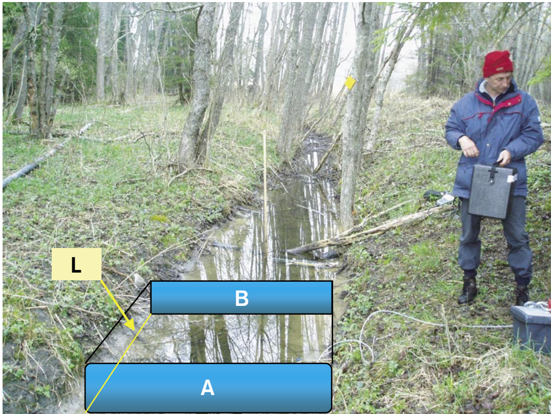
Figure 4-3. Schematic presentation of method for estimating water runoff in running natural waters. Sampling point PFM000073 (Söder Bredviken).
