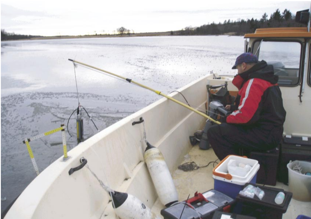
Figure 4-2. Measuring a profile (PFM000064) in the ice covered Baltic Sea with the multiple sonde (YSI 6600 EDS), December 15, 2003.
