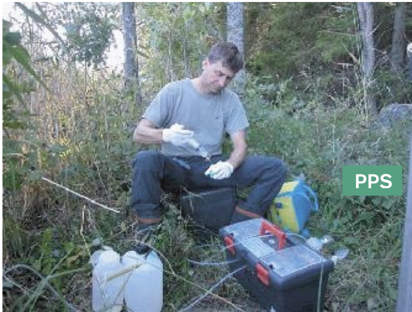
Figure 4-1. Sampling of surface water in the field. In front of picture, the peristaltic pumpsystem (PPS).
