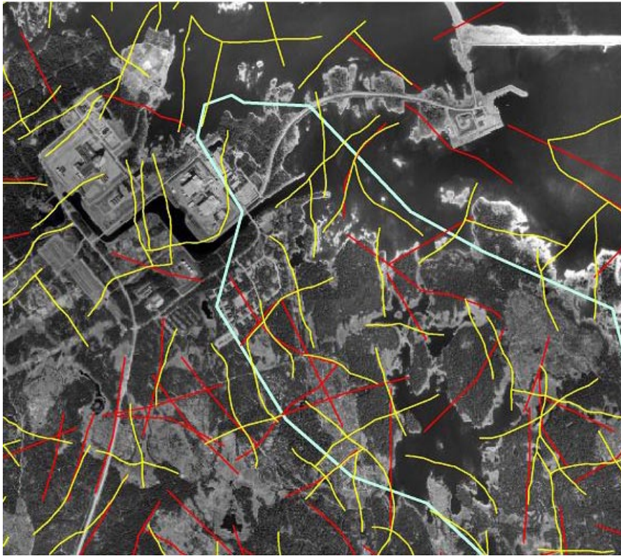
Figure 5-3. Linked lineaments 500–1,000 m superimposed on a mosaic of grey scale orthophotos. The primary (GeoVista) interpretation in yellow and the alternative (GTK) interpretation in red.
