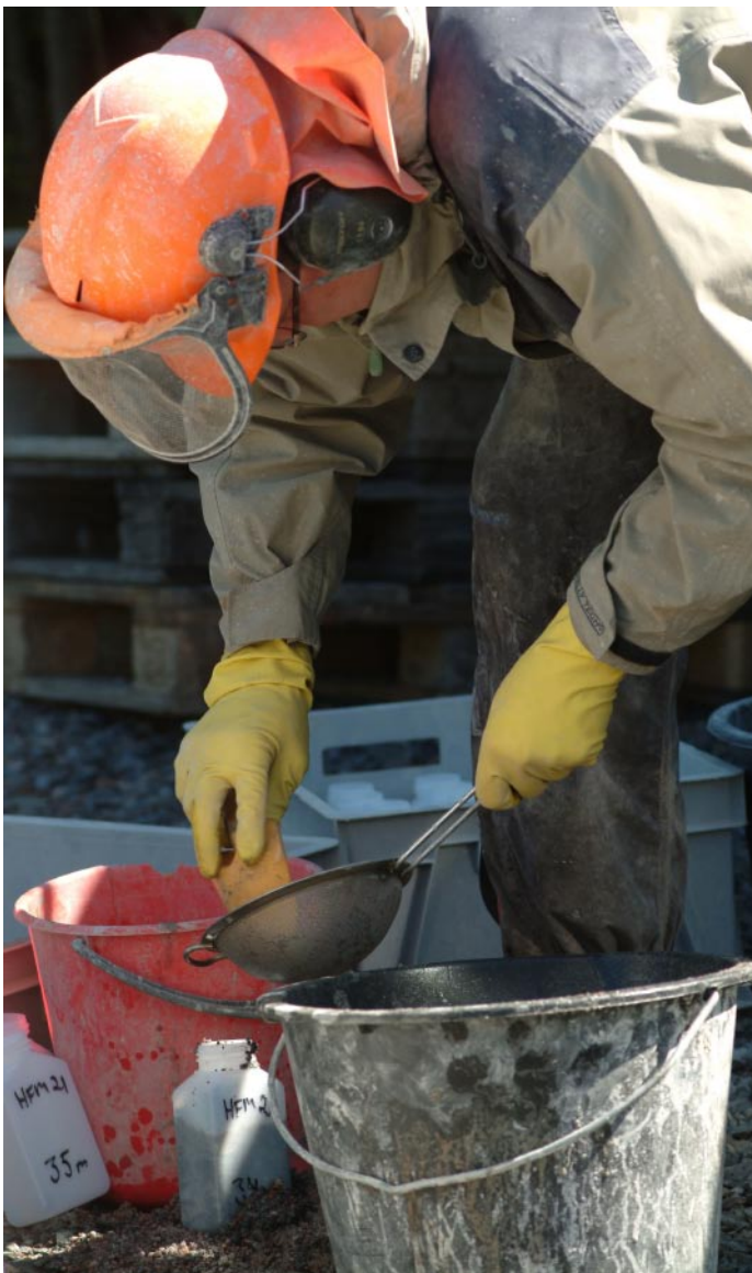
Figure 4-2. Samples of soil and drill cuttings were collected in plastic boxes and groundwater in small bottles.
