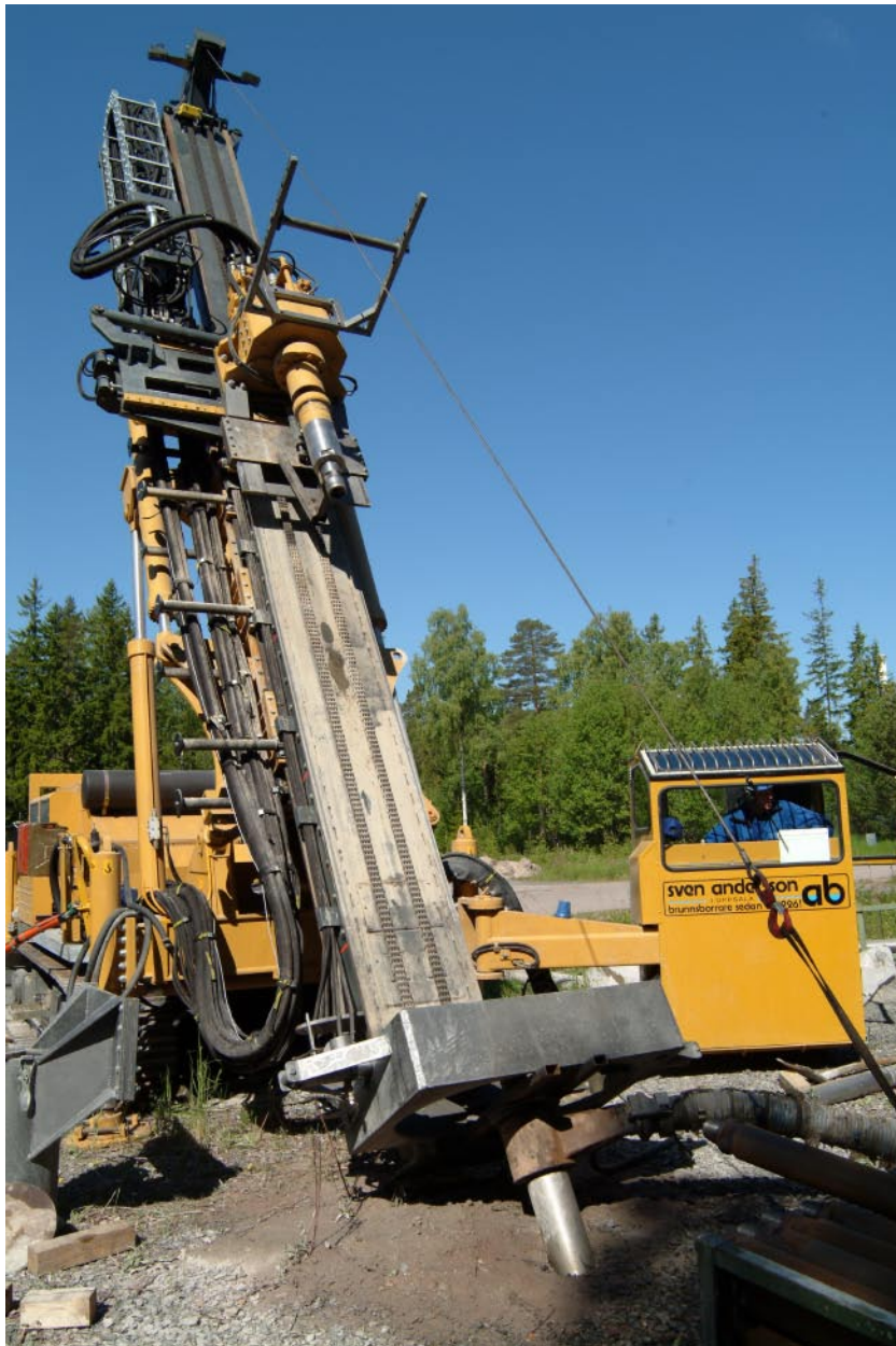
Figure 3-1. The Comacchio 1500 S percussion drilling machine in action on borehole HFM21 at DS7.
