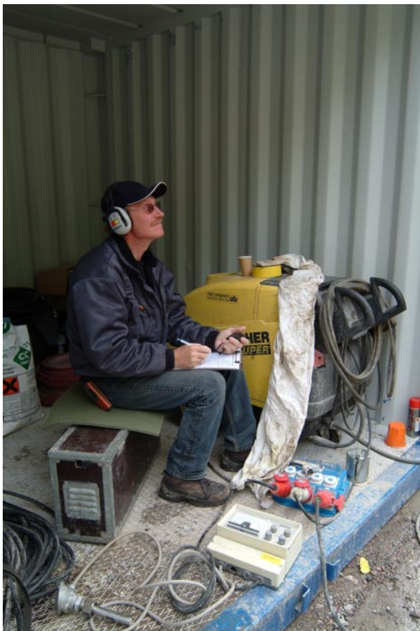
Figure 3-4. Manual measurements of drilling penetration rate were performed with a carpenter's rule and a stop watch in order to check the results provided by the automatic MWD-system.
