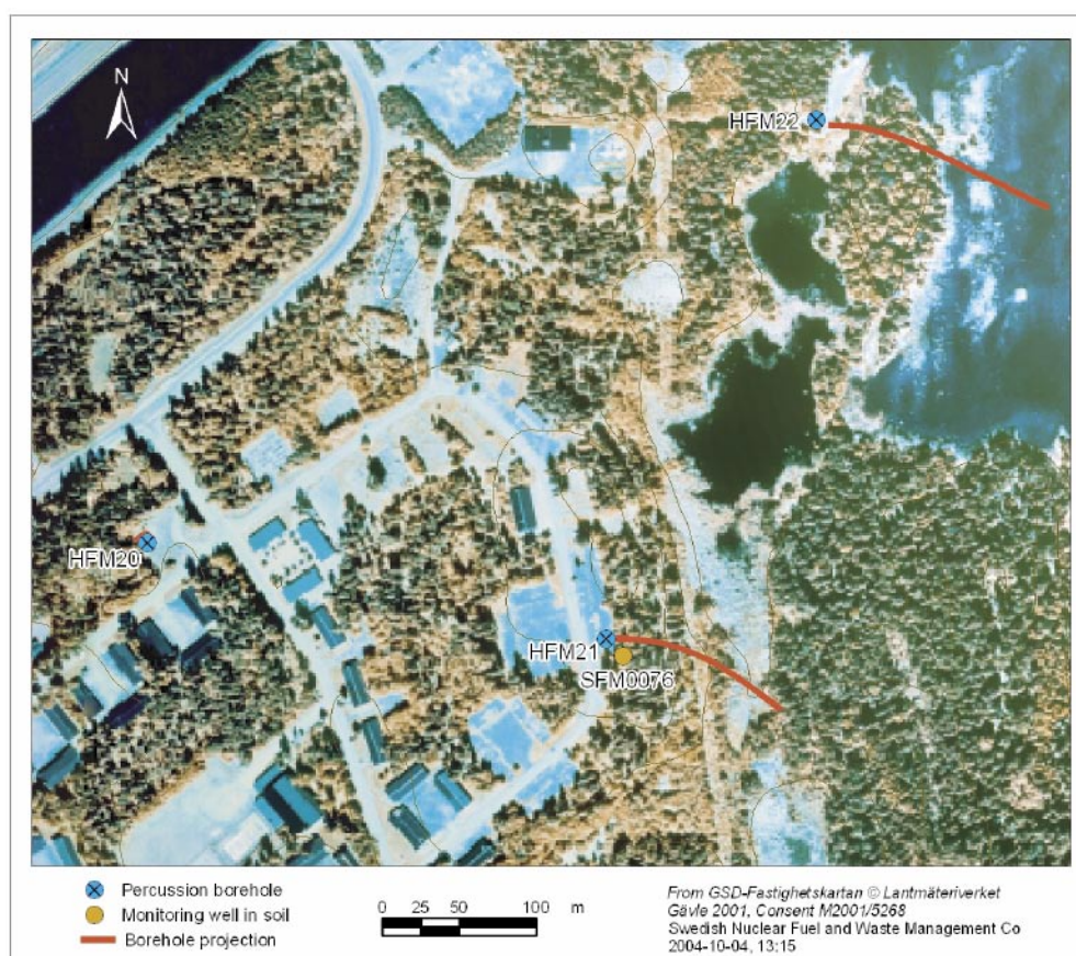
Figure 1-2. Borehole locations at and nearby drill sites DS7 (HFM21 and SFM0076) and DS8 (HFM22). Borehole HFM20 is situated about 300 m WNW of drill site DS7. The projections of inclined boreholes (all but SFM0076) on the horizontal plane at approximately the ground level (top of casing) are shown.
