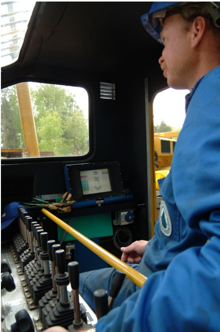
Figure 3-3. A D-MON logger system for measurements while drilling is mounted close to the control panel within the pilot house of the drilling machine.
