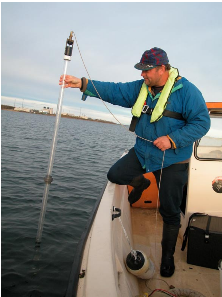
Figure 3-1. Sampling of sea water phytoplankton with a Ramberg rör at sampling point PFM000062.
