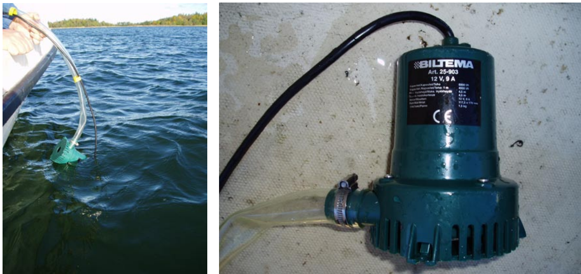
Figure 4-1. Submersible pump and a plastic hose.
