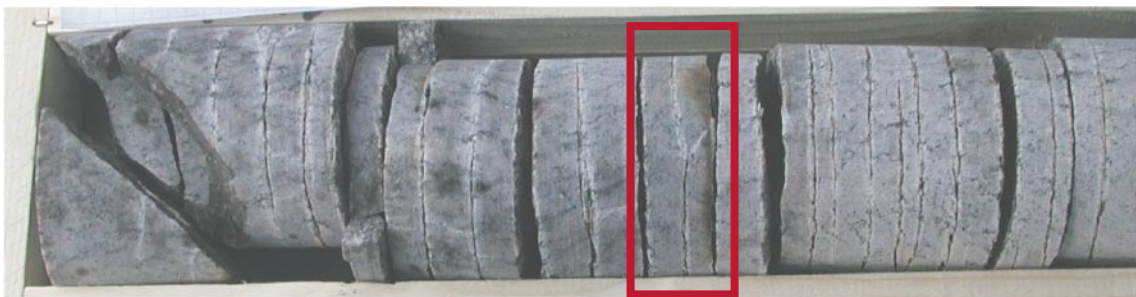
Figure 4-4. Overcore sample from test no 2:5:1, with the rock sample used for thin section preparation marked with a red rectangle.
