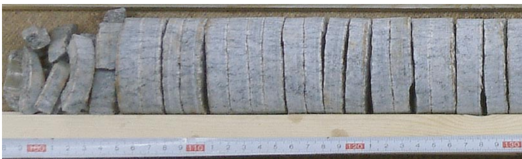
Figure 4-1. Photo of observed core discing in overcore sample for stress measurement no 2:10:1 (474.25 m depth).
