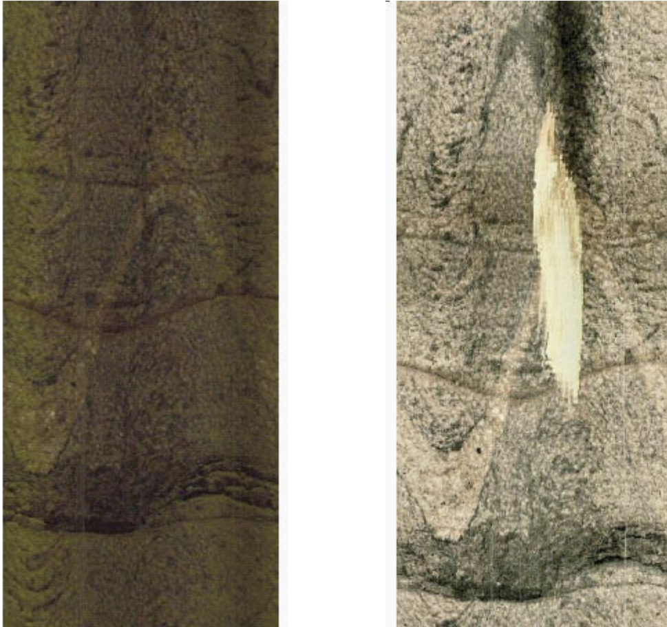
Figure 5-2. BIPS Images (left from June 2004, right from January 2005) from a 1 m section around 26 meter illustrating the improved quality between the two measurements.
