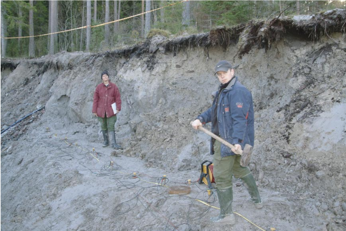
Figure 4-1. Execution of refraction seismic measurements on top of the compact moraine that occurs in the western trench. The geophone separation is 1 m.
