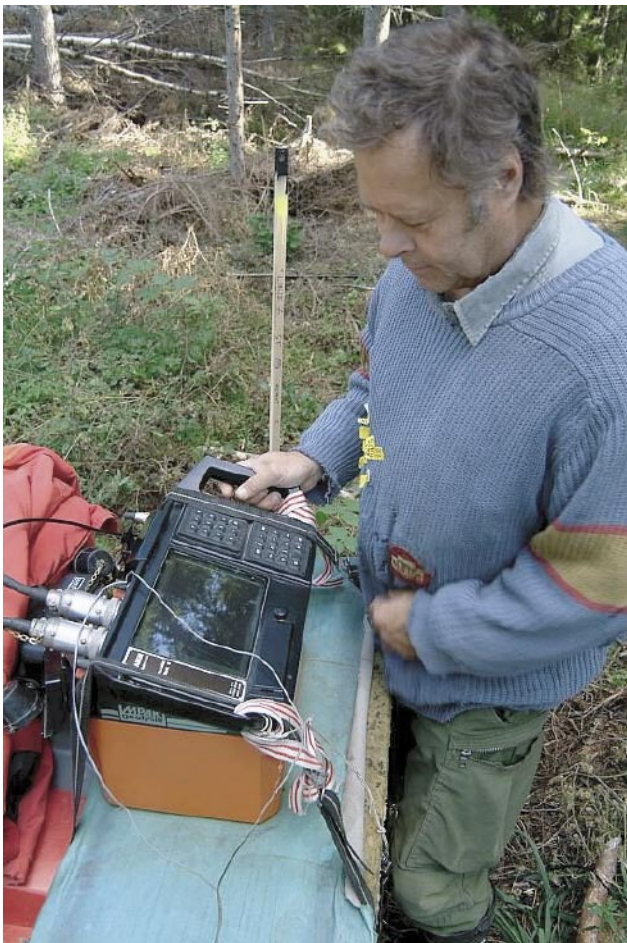
Figure 3-1. The seismograph used for refractions seismics.
