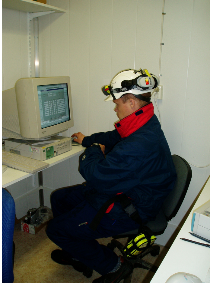
Figure 6-2 All pressure transducers are connected to the HMS system. In the G-tunnel is a computer in the HMS system where logging frequencies easily can be changed.
