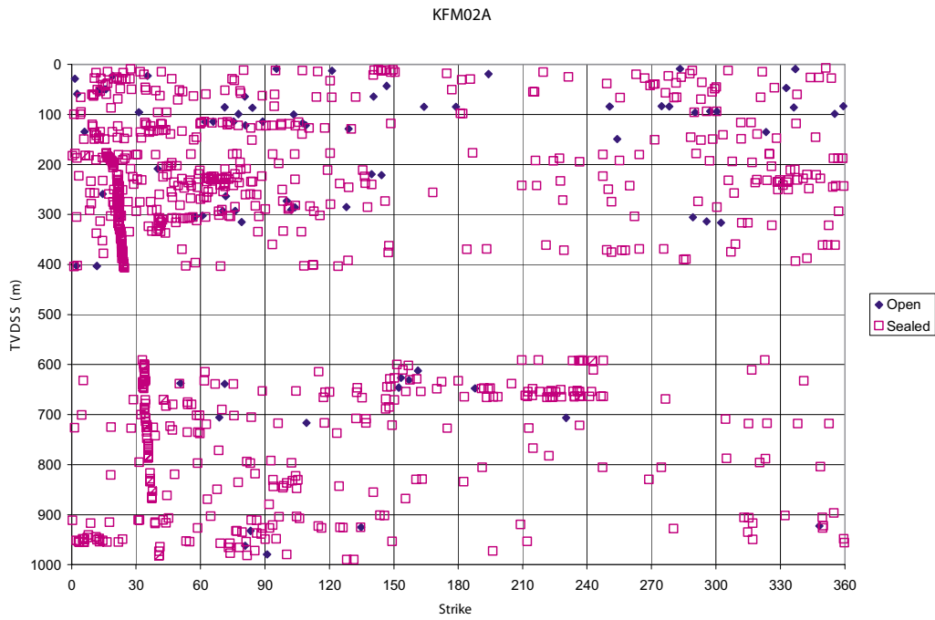
Figure 3. Variation of fracture strike with TVDSS, cored borehole KFM02A, open and sealed fractures.
