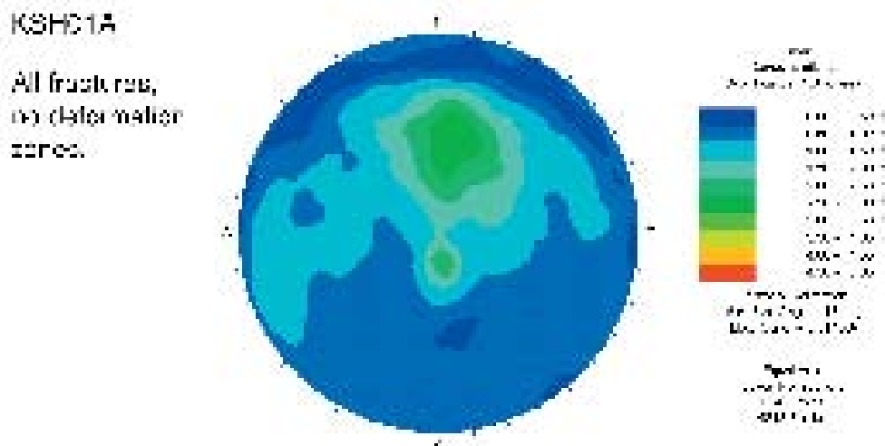
Figure 5-35. Equal area, lower hemisphere projection of contoured poles to fracture planes in borehole KSH01A (fractures associated with interpreted deformation zones excluded).
