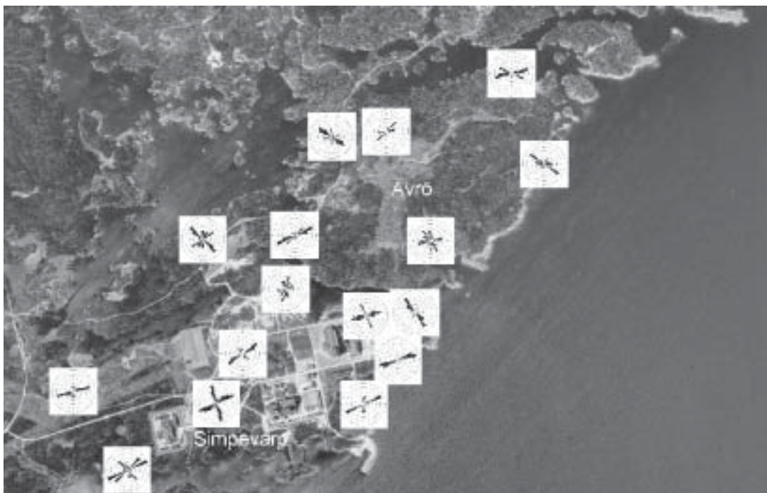
Figure 5-32. Orthophoto with diagrams showing fracture strike and frequency for fractures dipping 45 degrees or more at each outcrop.
