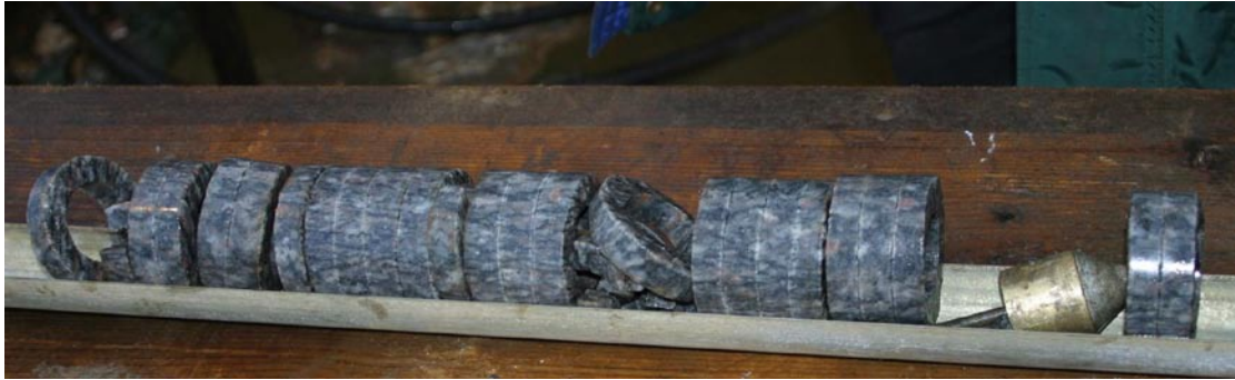
Figure 5-5. Example of core discing after stress relief of overcored rock sample from KFM01B.
