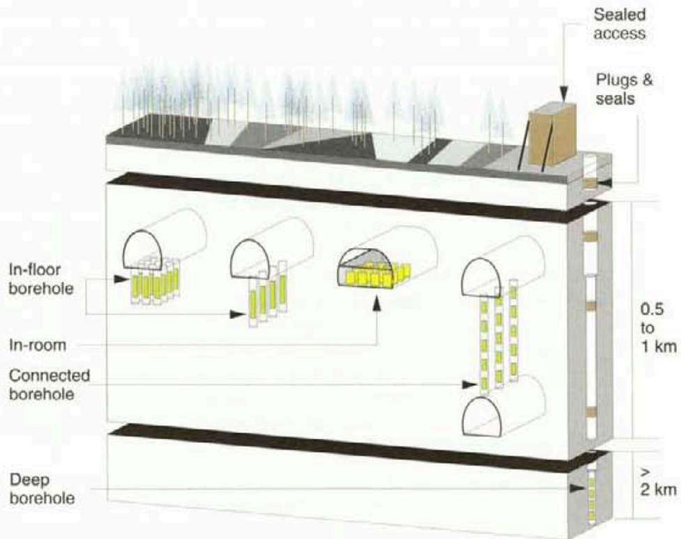
Figure 1-2 Waste container deposition options being considered for repositories in granite by member countries of the Stripa Project.
