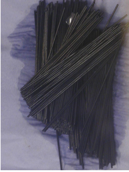
Figure 9. Condition of specimens on completion of corrosion experiments: LHS: Cell 7 Allard groundwater, 11 Gray hr -1 at 30°C, RHS: Cell 1, Bentonite-equilibrated groundwater, 11 Gray hr -1 at 50°C.
