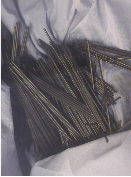
Figure 9. Condition of specimens on completion of corrosion experiments: LHS: Cell 7 Allard groundwater, 11 Gray hr -1 at 30°C, RHS: Cell 1, Bentonite-equilibrated groundwater, 11 Gray hr -1 at 50°C.
