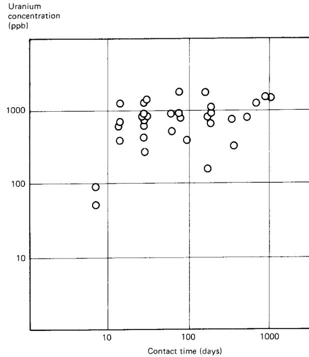
Figure 10-1. Measured concentrations of uranium in leach solution centrifugates as a function of time.
