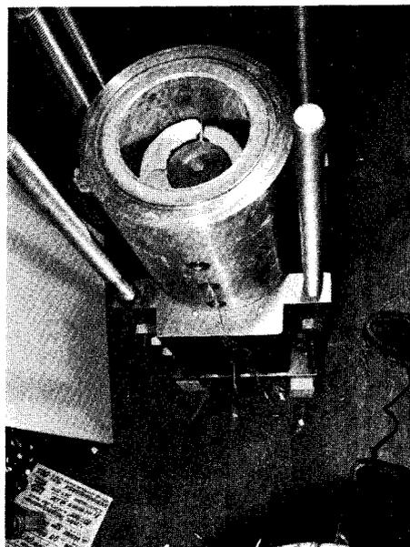
Figure 11-4b. The upper part of the deposition hole is mounted. Some of the cables from the strain gauges and the pressure transducers can be seen.
