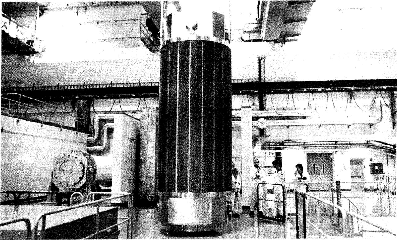
*Figure 3-3. Transport flask in the fuel reception building at CLAB.*
