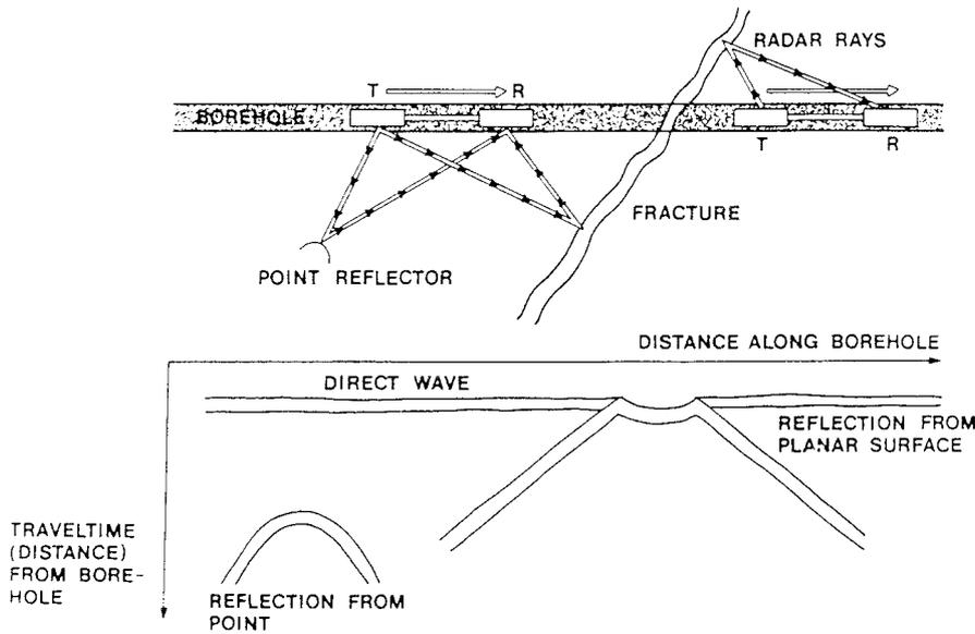
Figure 16-1. The principle of borehole reflection radar and the patterns generated by plane and point reflector.
