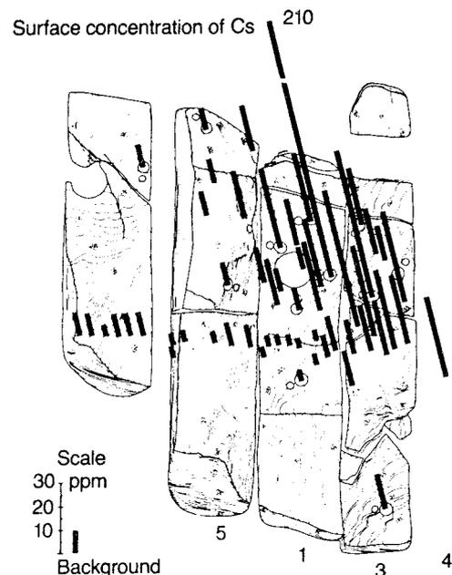
Figure 16-2. Distribution of Cesium around the injection point in the tracer experiment along a single fracture.
