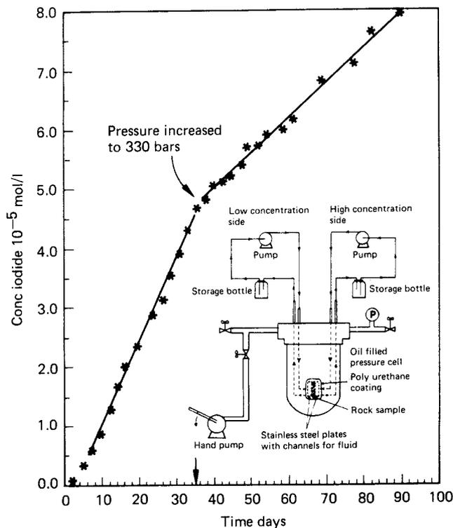
Figure 12-6. Iodide diffusion through a biotite gneiss sample from the investigation site Svartboberget. The experiment was started at atmospheric pressure which was increased to 330 bar after 35 days.
