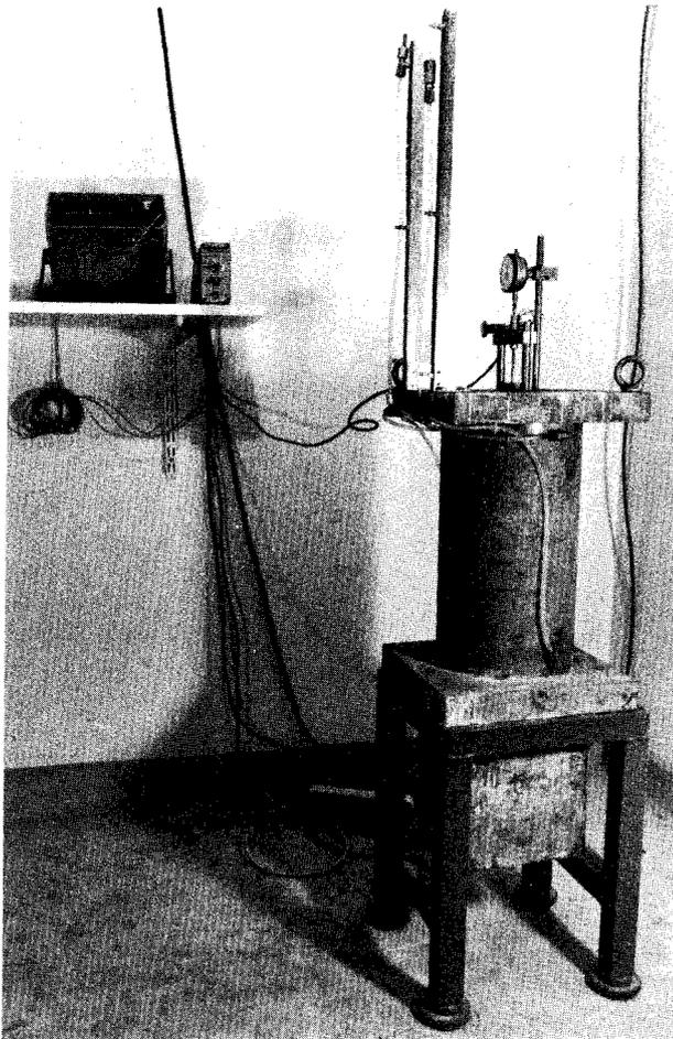
Figure 11-2. Experimental setup in climate chamber. The settlement reading is made by use of an electronic transducer with a nominal accuracy of  $10^{-7}$  m.
