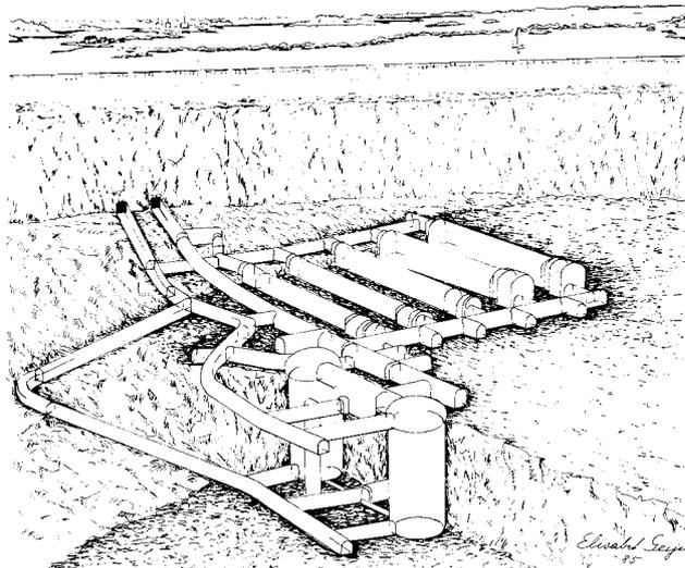
Figure 5-1. Overview of tunnels and storage chambers in SFR.
