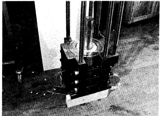
Figure 11-4a. The copper canister and the compacted bentonite placed in the lower part of the "deposition hole".
