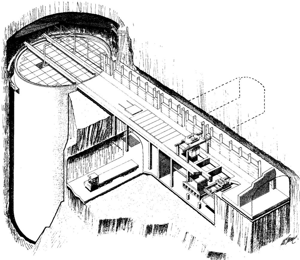
Figure 5-3. The Silo repository with remote handling of waste packages.
