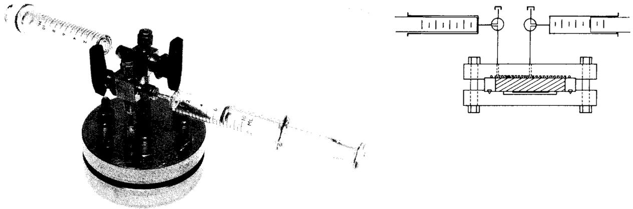
Figure 12-7. Equipment for measuring the hydrogen production in alpha irradiated compacted water saturated bentonite ( $2.1 \text{ g/cm}^3$ ). The radiation source is  $^{241}\text{Am}$  with an active surface diameter of 25 mm. The nominal activity is 30 MBq.
