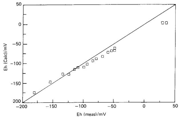
Figure 12-3. Eh calculated for the sulphide/sulphur system compared to Eh measured with a platinum electrode in the ground surface equipment. The water is pumped up to the ground surface.
