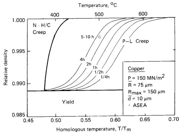
Figure 10-5. Density-temperature diagram for hot isostatic pressing of copper.
