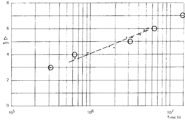
Figure 11-3. Settlement of model canister. Crosses represent recorded settlement while rings are predicted settlement for specific time values.
