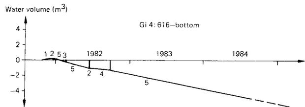
Figure 12-1. The variation in water budget in different groundwater sampling sections in the borehole Gideå 4 due to 1) drilling, 2) gas-lift pumping, 3) hydraulic testing, 4) sampling and 5) open hole effect. Increasing values means inflow to the rock from the borehole. The calculations are based on measurements of hydraulic conductivity.
