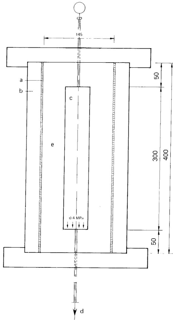
Figure 11-1. Schematic picture of model canister (c) embedded in highly compacted bentonite (e) with a bulk density of about  $2.1 \text{ t/m}^3$  in a water saturated state. b is a steel container and a filter for water saturation. d is a dead load of 80 kg.
