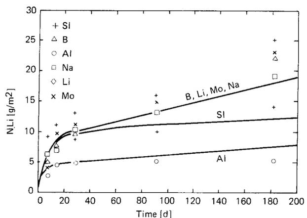
Figure 10-3. Comparison of leach results of JSS glass in deionized water (MCC-1 test,  $90^\circ C$ ,  $10 m^3$ ) with the computer simulation (solid lines).
