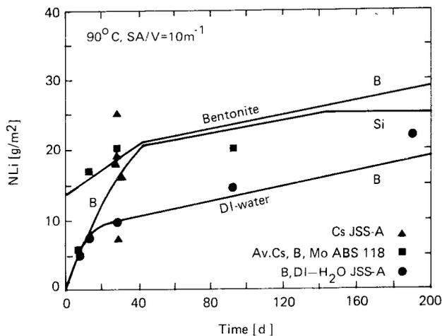
Figure 10-4. The effects of bentonite on glass leaching: model (solid lines) and experiment.
