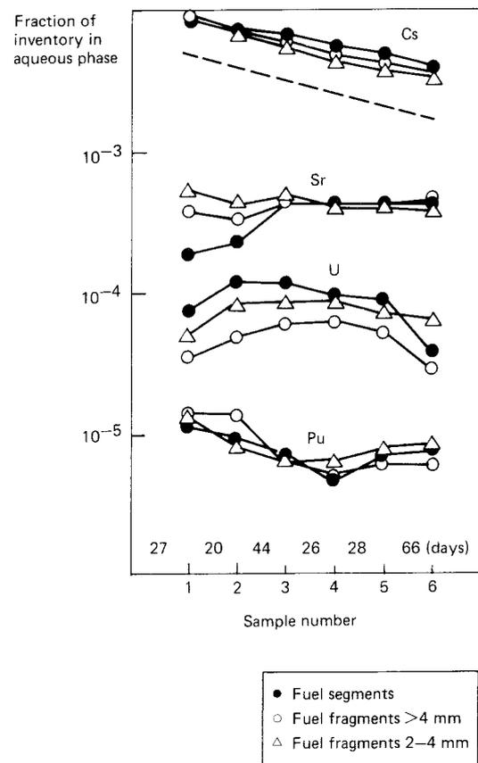
Figure 10-2. Replenishment experiments: Variation of leach fraction with successive replenishment. (Fuel segments are cut from a fuel pin and include both fuel and zircalloy cladding. Fuel fragments consist of spent fuel without cladding.)
