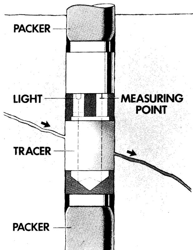
Figure 13-3. Dilution probe for measurement of groundwater flow.
