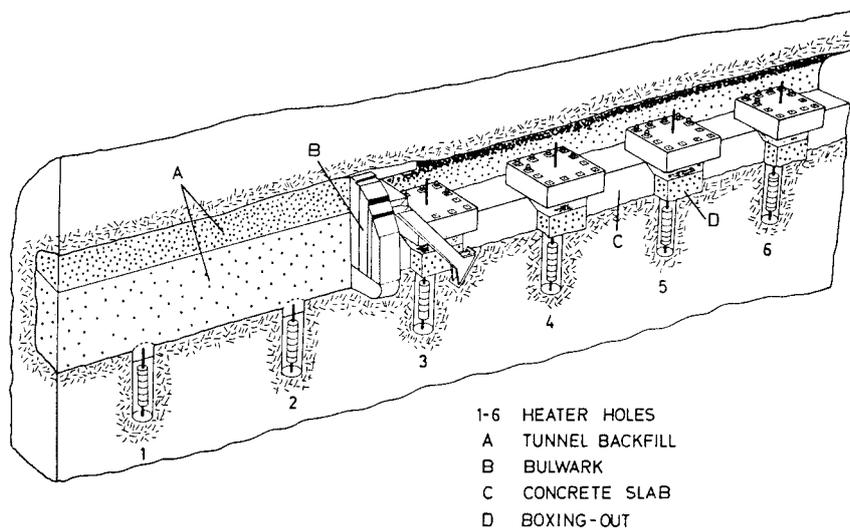
Figure 16-4. Main features of the Buffer Mass Test.
