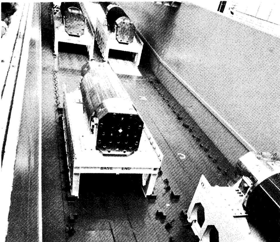
*Figure 4-2. Transport flasks in the cargo hold of M/S Sigyn.*
