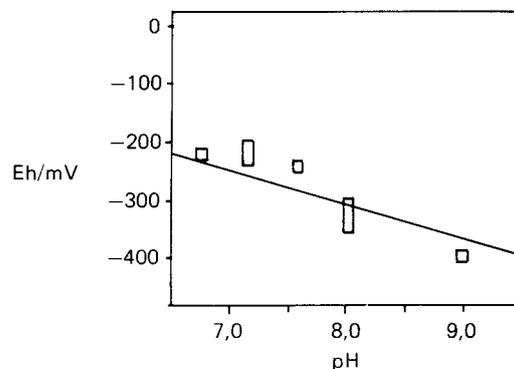
Figure 12-4. Eh and pH values of groundwater measured in situ with the downhole equipment. The bars indicate the maximum variation of the Eh values measured simultaneously with platinum, gold and glassy carbon electrodes. The line corresponds to the redox equilibrium in the magnetite/hematite system.
