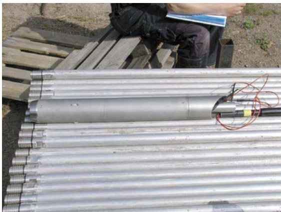
Photo 5. Positioner, bottom end of down-hole string.
