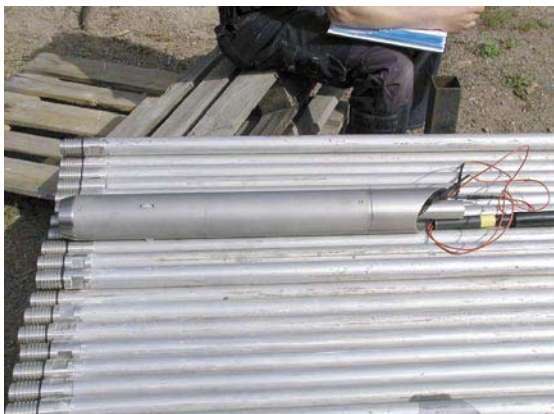
Photo 5: Positioner, bottom end of down-hole string.
