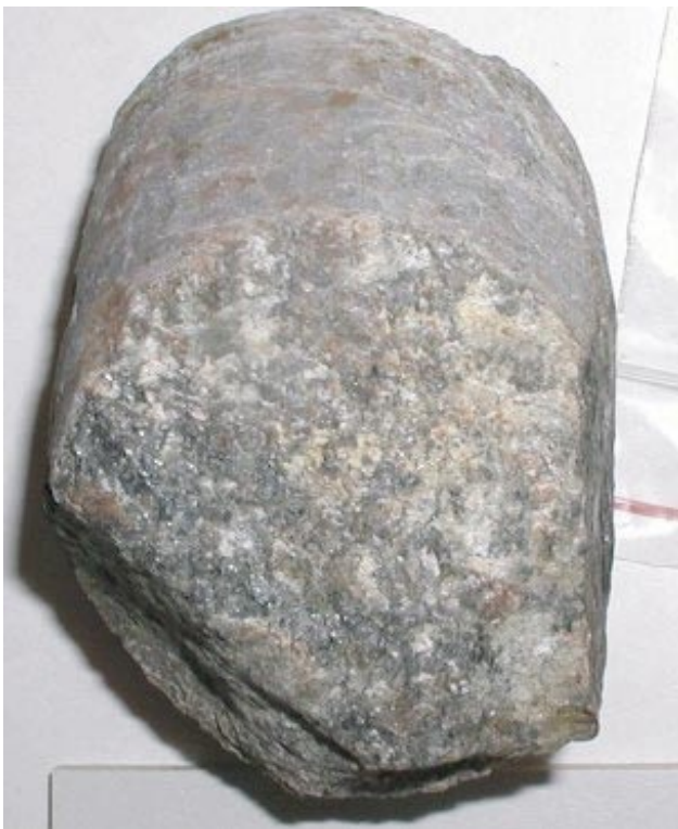
Figure A-41. Open fracture with a mixture of quartz, albite, K-feldspar, chlorite/corrensite and calcite. The diameter of the drill-core is c 5 cm (KFM02A 423.65–423.70 m).
