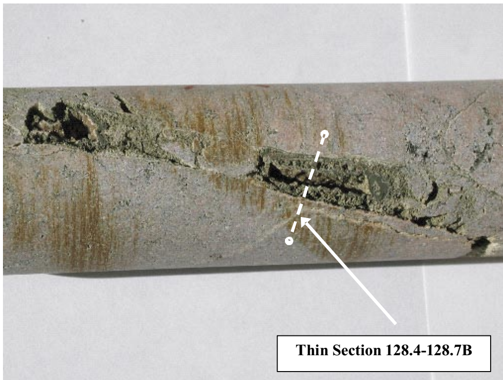
Figure A-7. Mineral filled fracture. The diameter of the drill-core is c 5 cm (KFM01A 128.4–128.7 m (B)).
