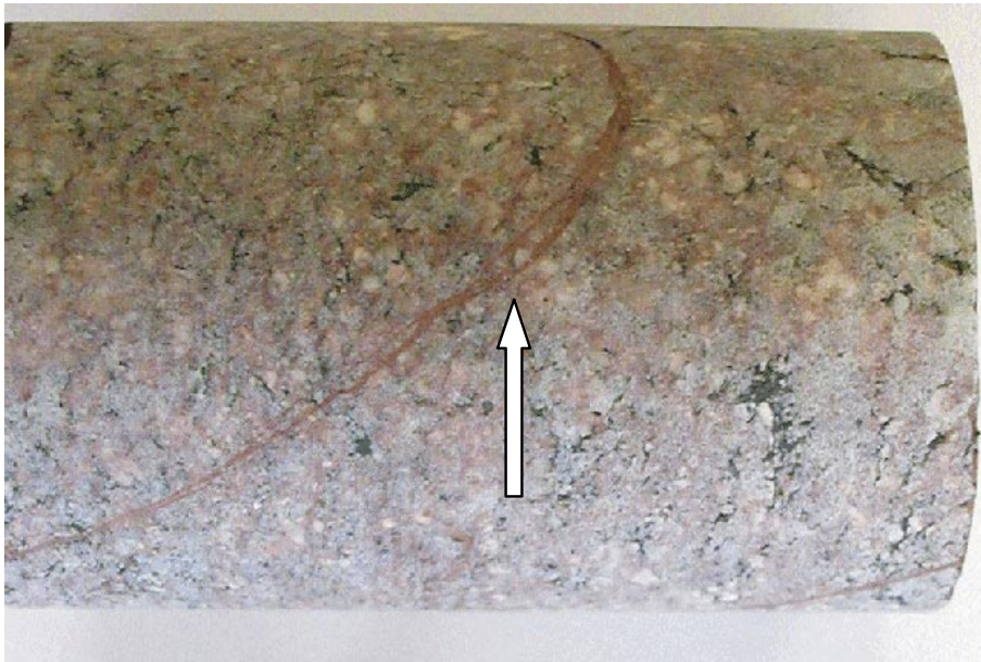
Figure 5-5. Fracture filled with adularia that is brick coloured due to micro-grains of hematite. Some calcite is also present in the fracture. The diameter of the drill-core is c 5 cm. (KFM03A 184.34–184.50 m).
