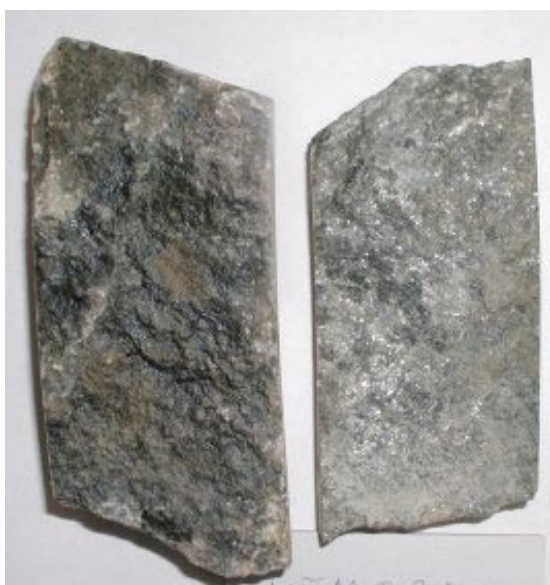
Figure A-46. Open fracture with apophyllite (the shiny mineral) and corrensite (the black mineral). The diameter of the drill-core is c 5 cm (KFM02A 893.45–893.65 m).
