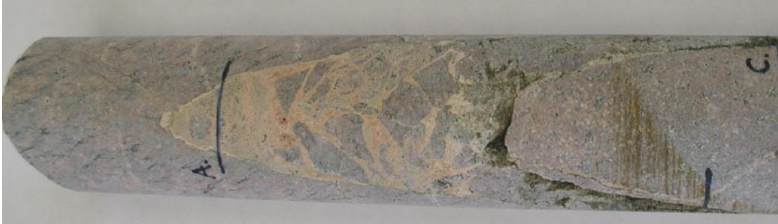
Figure 5-3. Laumontite sealed breccia (Generation 3) cut by a fracture filled with adularia (Generation 4 or possibly a very late phase of Generation 3). The diameter of the drill-core is c 5 cm (KFM01A 124.4–124.8 m).
