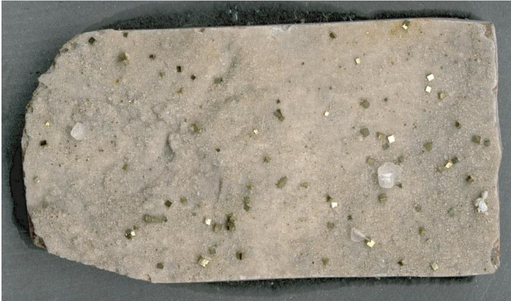
Figure 5-6. Calcite and pyrite crystals (Generation 5) on top of a quartz coated fracture surface (Generation 4). Length of photograph is 2.5 cm (KFM01A 267.0 m).
