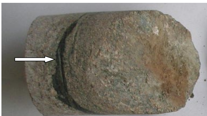
Figure A-30. Fracture filled with altered prehnite. The diameter of the drill-core is c 5 cm (KFM02A 111.0–111.15 m).
