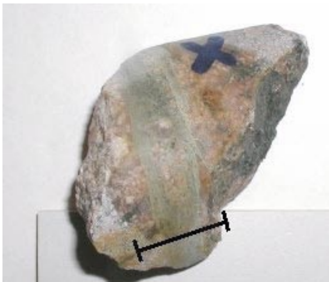
Figure A-44. Epidote filled fracture, partly mylonitized, cut by open fracture. The diameter of the drill-core is c 5 cm (KFM02A 516.60–516.65 m).
