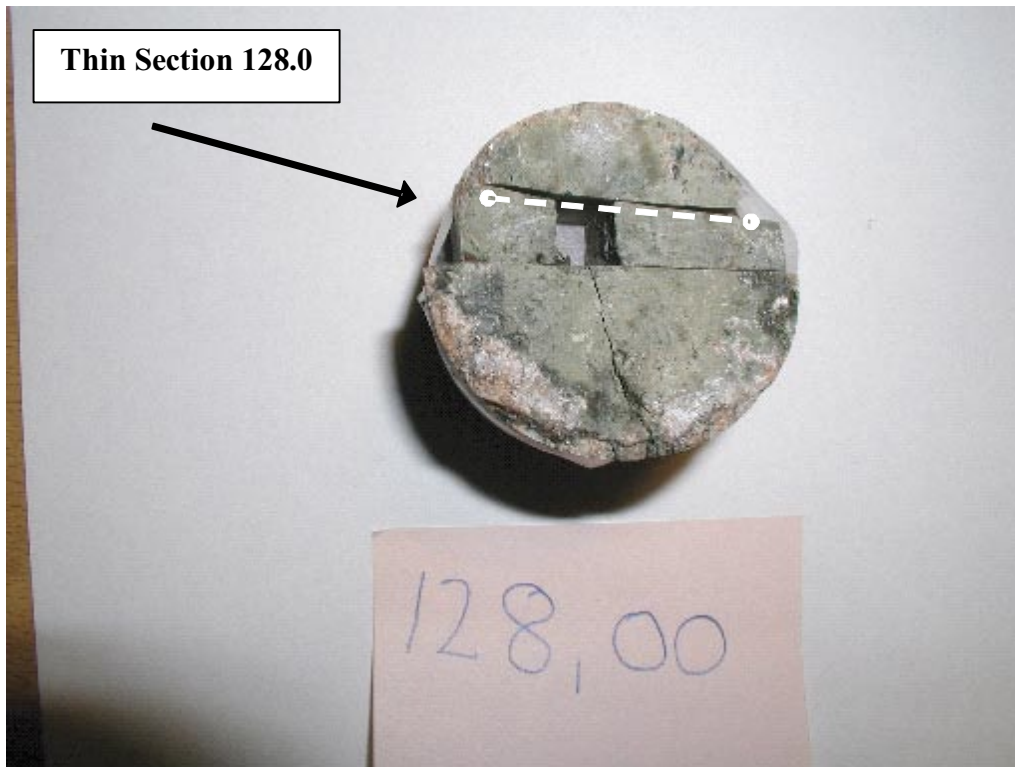
Figure A-5. Fracture surface with thin quartz and adularia coating. The diameter of the drill-core is c 5 cm (KFM01A 128.0 m).
