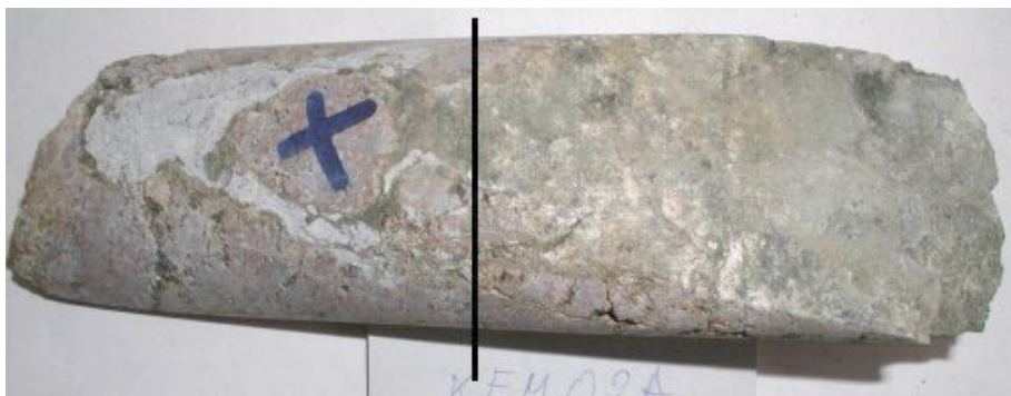
Figure A-38. The wall rock is cut by a white, mainly calcite-sealed fracture. The drill-core is 5 cm in diameter (KFM02A 422.30–422.40 m).
