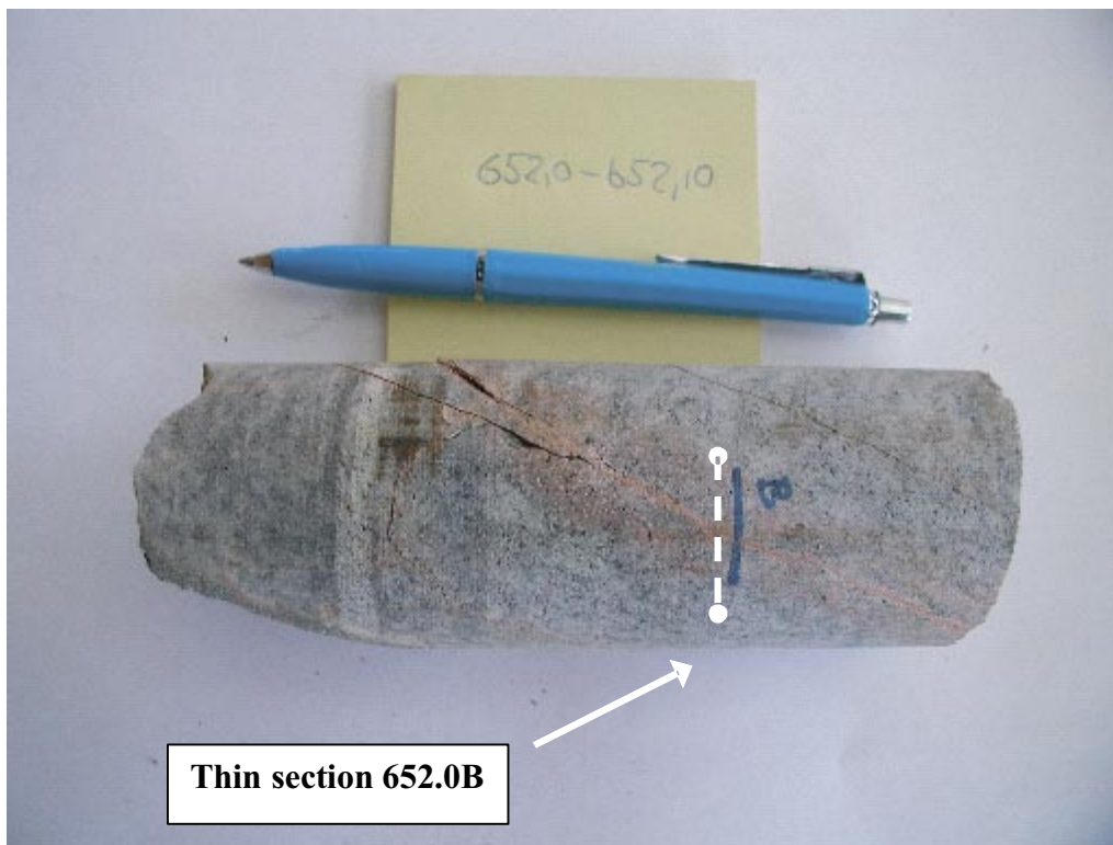
Figure A-25. Laumontite sealed thin fracture with hematite and later quartz (KFM01A 652.0 m (B)).
