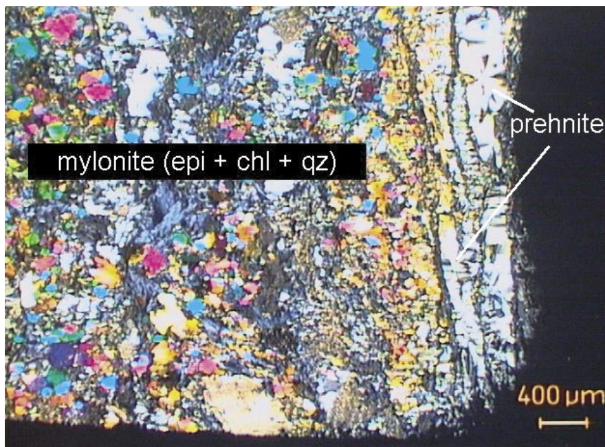
Figure 5-2. Mylonite with epidote, chlorite and quartz (Generation 1) on which prehnite (Generation 2) has crystallized. (Microphotograph KFM03A 451.85–451.90 m).
