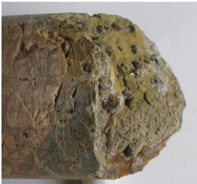
Figure A-34. Open fracture coated with small idiomorphic quartz crystals under larger idiomorphic pyrite crystals. The diameter of the drill-core is c 5 cm (KFM02A 171.40 m).
