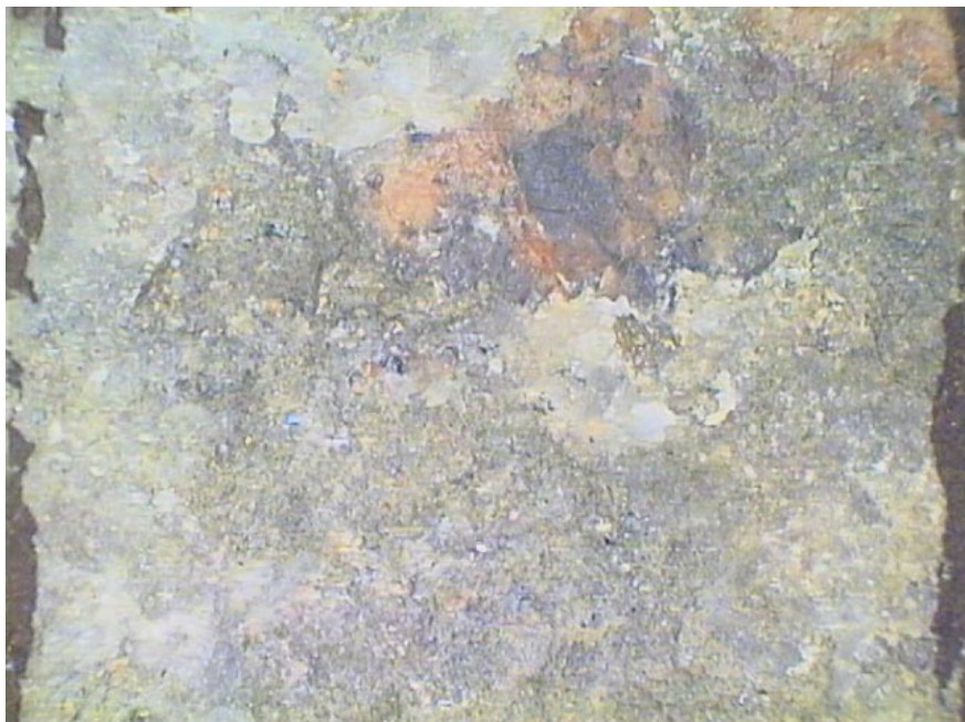
Figure A-37. The white mineral is calcite and the small green-coloured minerals are feldspar. The illite is not visible in this scale. The base of the figure is c 2 cm (KFM02A 403.13 m).
