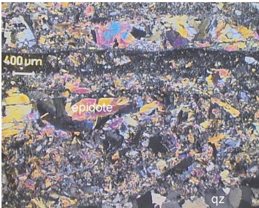
Figure 5-1. Epidote mylonite-cataclasite. The fine-grained matrix consists of epidote. (Microphotograph KFM02A 516.60–516.65 m).
