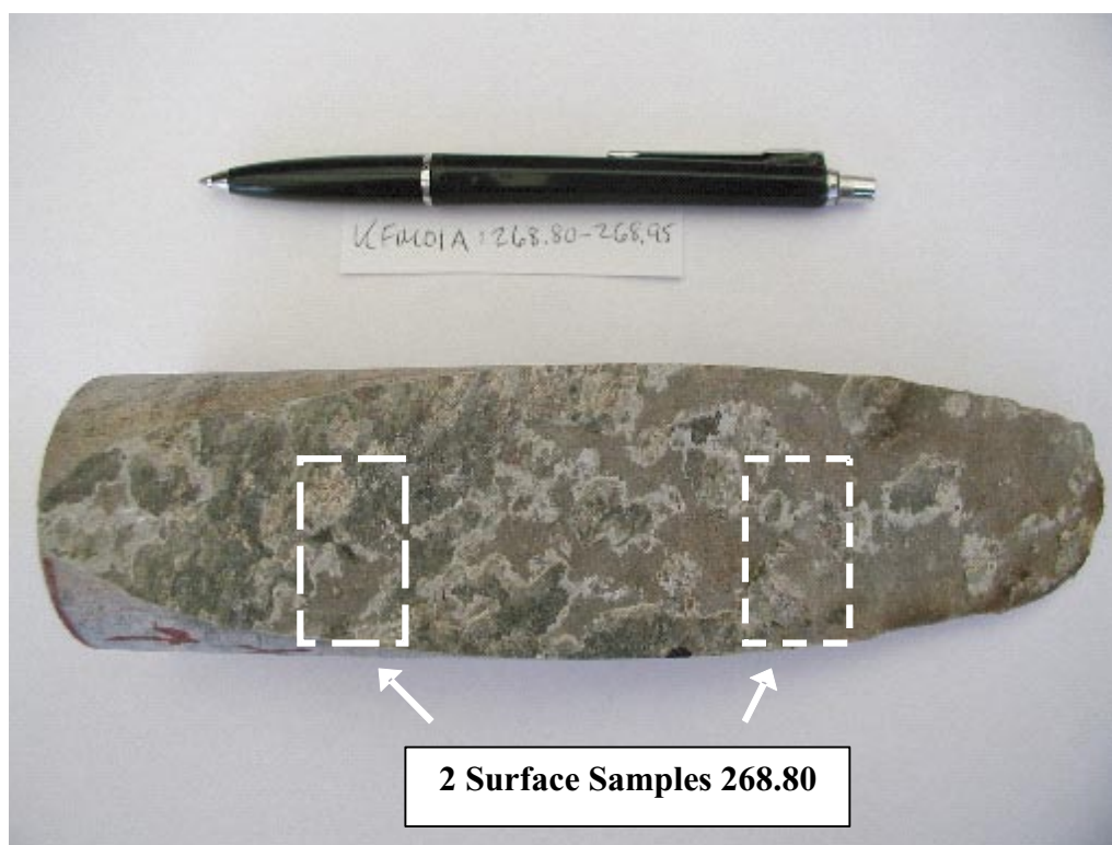
Figure A-19. Quartz covered fracture surface with pyrite, barite and mixed-layer clay (KFM01A 268.8 m).
