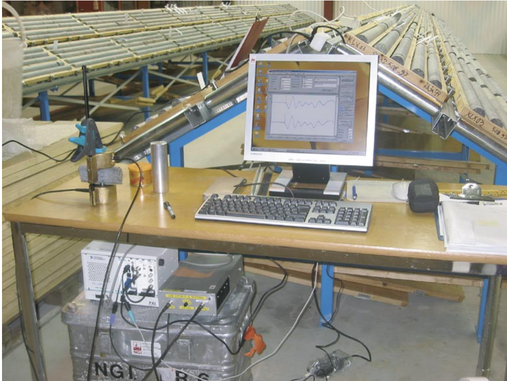
Figure 3-2. NGI's equipment set-up for measuring acoustic P-wave travel time transverse borehole core.
