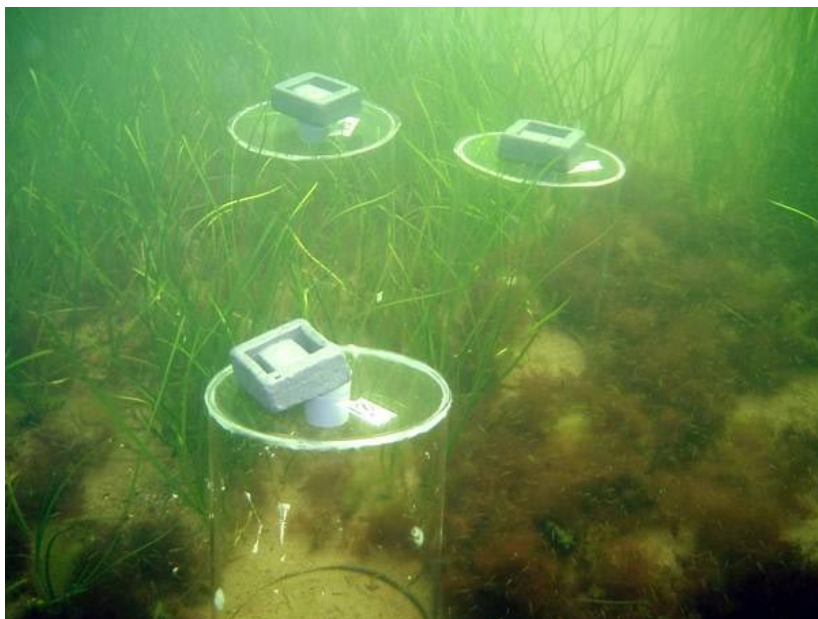
Figure 3-4. Investigation setup for production and respiration estimation in aquatic environments.
