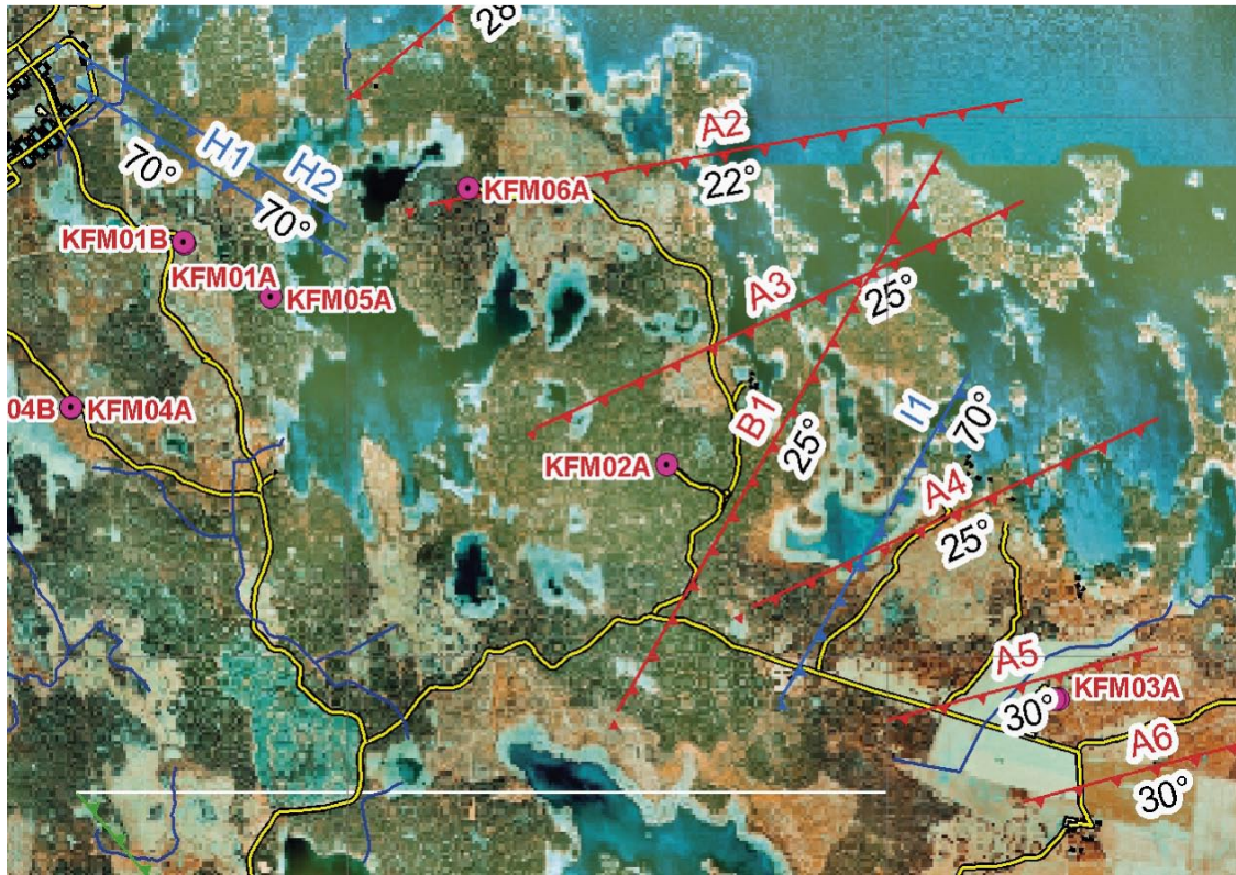
Figure 3-18. Intersection of reflectors with the ground surface, interpreted from seismic reflection surveys. These reflectors, which probably represent fracture zones, are likely to be of crucial importance for water transport through the southeastern part of the investigation area in particular.
