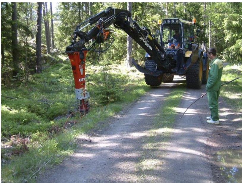
Figure A-10. Seismic survey with impact hammer.
