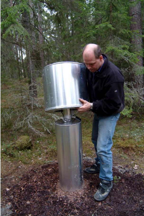
Figure A-2. Preparations for measurement of groundwater level in soil boreholes.
