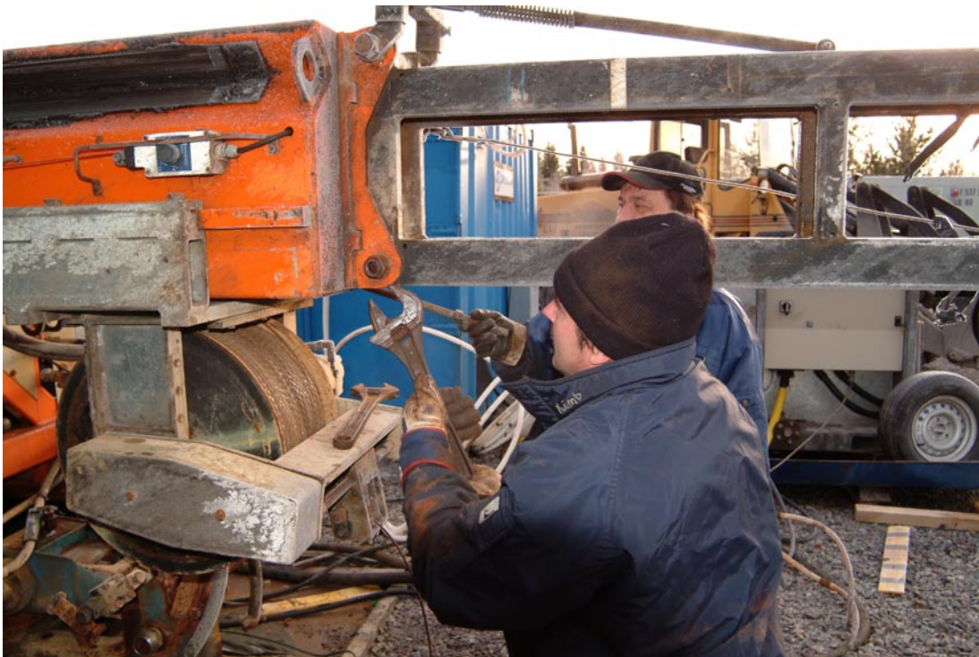
Figure 1-5. Core drilling outfit during mobilization on drilling site DS5.
