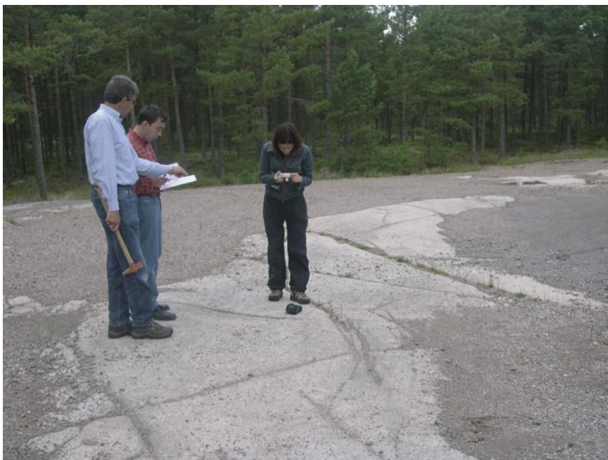
Figure 2-4. Photograph of the outcrop ASM000026 , which emphasizes the small density of small fractures in contrast with Figure 2-3.
