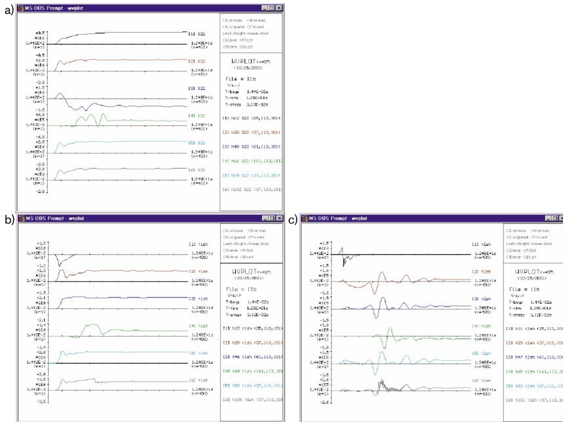
Figure A2b-10. (a) Models 11–16 – induced normal stress, (b) Models 11–16 – shear stress shT1 (s12), (c) Models 11–16 – shear stress shT2 (s23).
