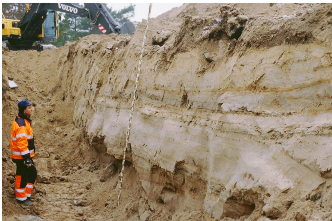
Figure A3-11. A trench, machine-cut during the Forsmark site investigations, Sweden, is studied for seismically induced liquefaction. The trench is c 80 m long, located on the eastern flank of the Börstilåsen Esker site investigations.
