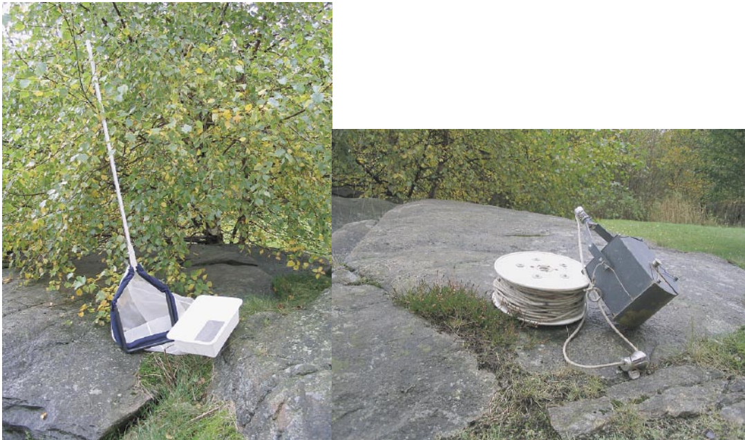
Figure 3-1. The hand net and sieve used in the littoral zone of the lakes and in the streams and the Ekman grabber used in the deeper parts of the lakes.
