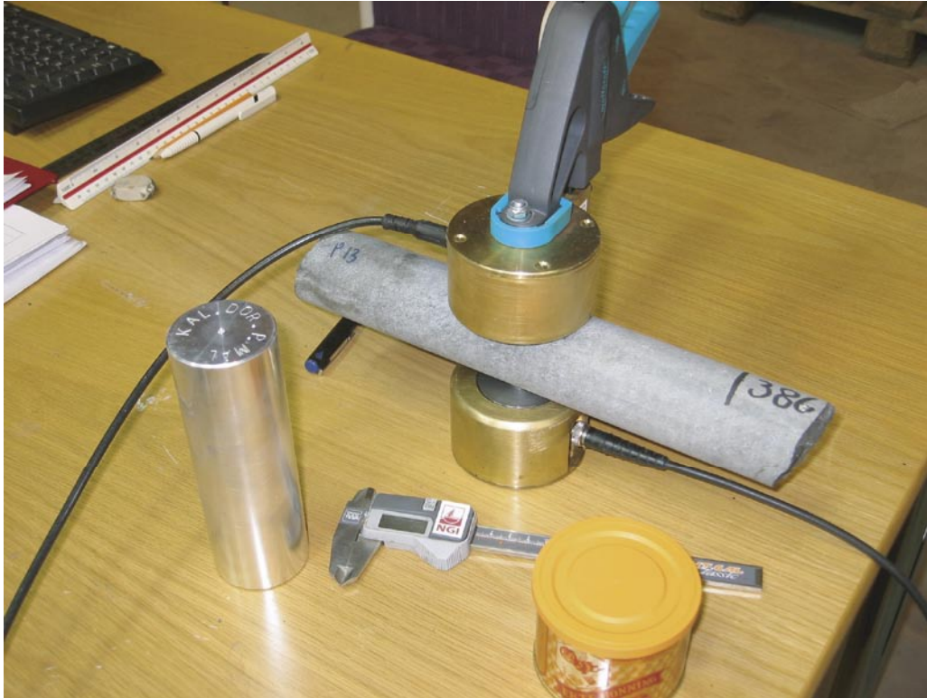
Figure 3-2. Detail of NGI's apparatus for measuring acoustic P-wave travel time transverse the drill core. The aluminium cylinder for calibration of the device is on the left.
