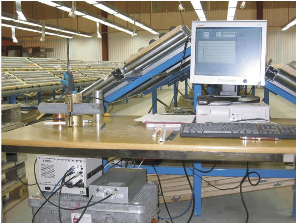
Figure 3-1. NGI's equipment set up for measuring acoustic P-wave travel time transverse the drill core.
