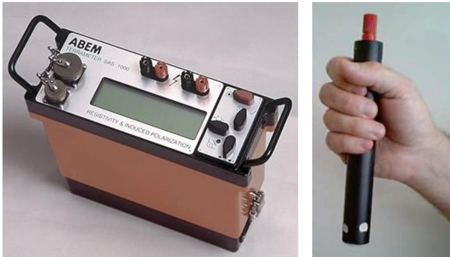
Figure 3-1. The Terrameter SAS 1000 (left) and a non-polarizable electrode (right).
