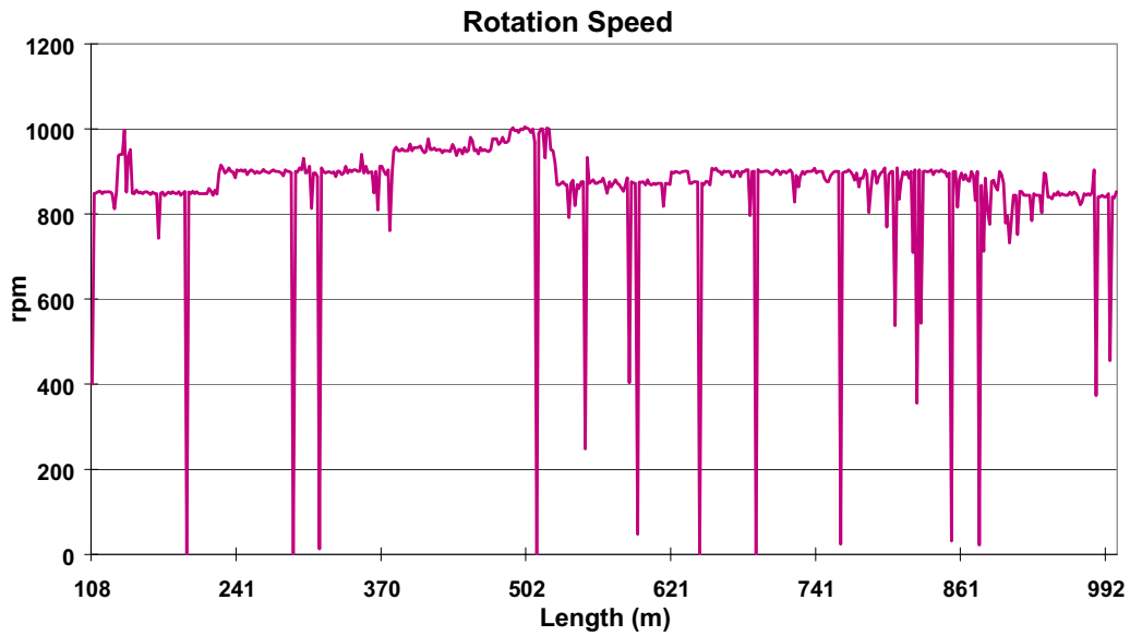
Figure 5-8. Rotation speed versus borehole length during drilling of borehole KFM04A.
