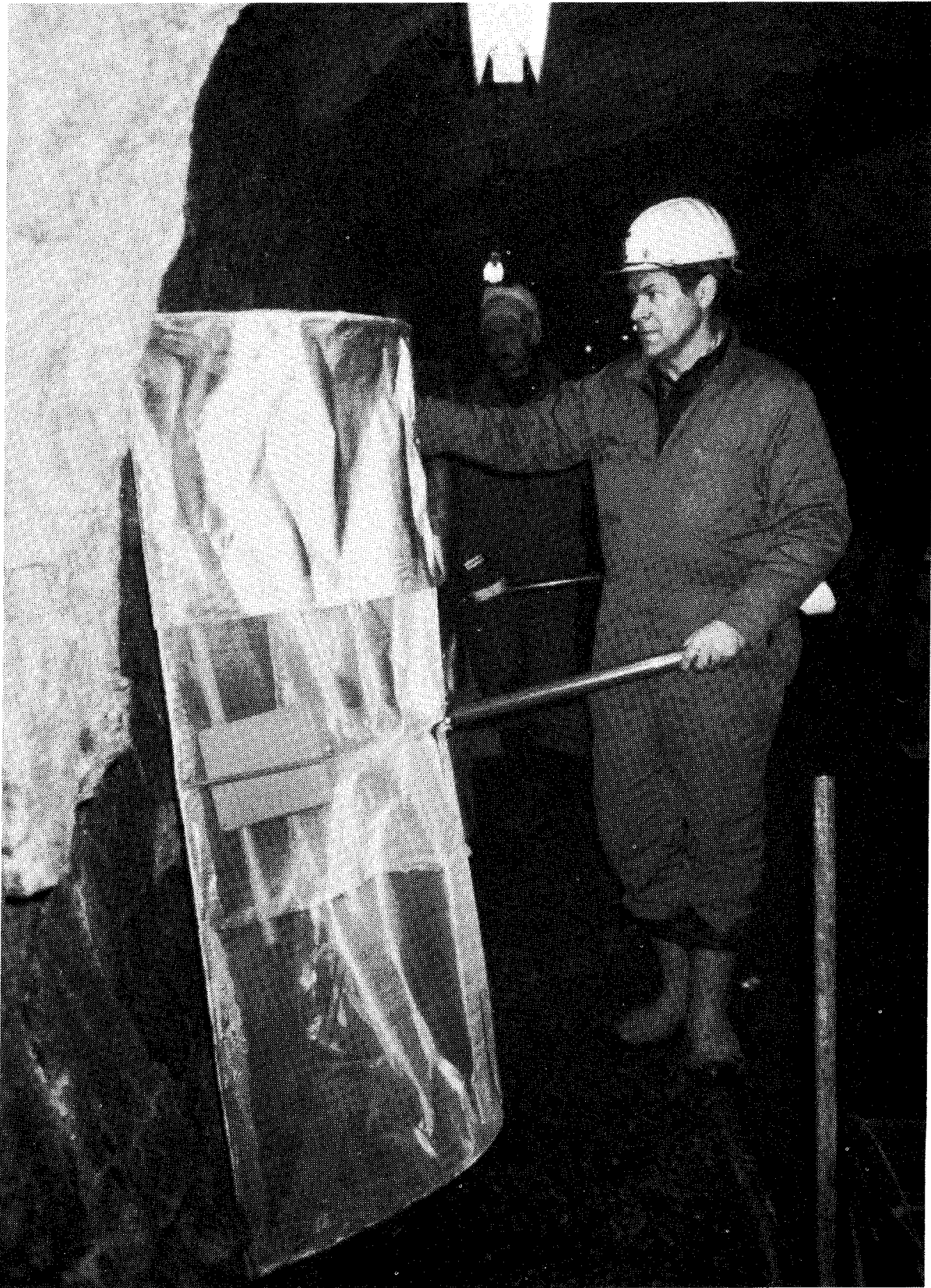
Figure 4.23 Metal net used as a screen to test the antennas.
