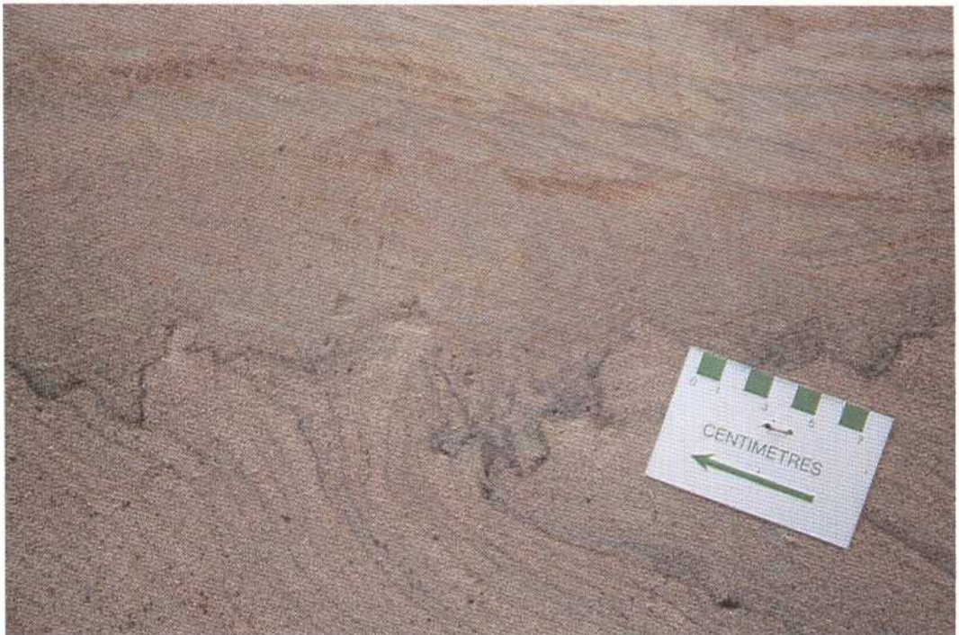
Figures 15 a and b. Disturbed 5-10 cm thick zone in cross-bedded deltaic sand at Slättheden (site 2). Note (gravitational) enrichment of heavy minerals and coarser grains along the strongly deformed contact between inclined, evenly bedded sand below and current-bedded sand above. The deformations are interpreted as possible effects of earthquake-induced liquefaction and dewatering during the build-up of the sequence. Photo: R.L. 1990.
