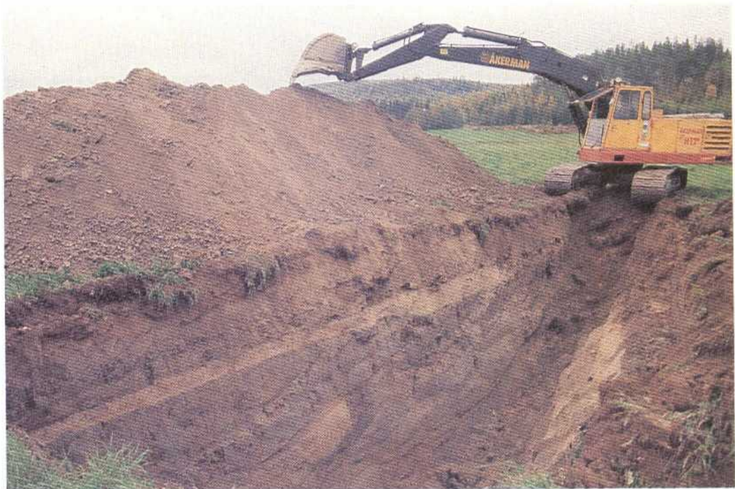
Figure 55. Trench dug through deformed sandy and silty glacial sediments covered by laminated (varved) silty clay at Botsmark some 50 km north of Umeå. The thick sand sheet between the clay and the deformed sediments below is interpreted to represent the fall-out from turbulent water in connection with earth tremor and faulting in the region. Photo: R.L. 1990.
