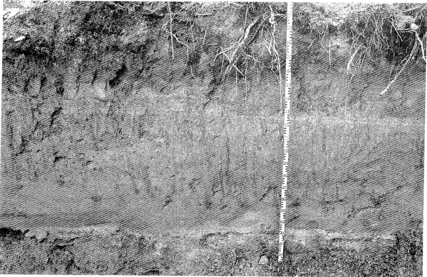
Figures 17 a, b and c. Deformed sediment sequence at the distal part of the delta deposits at Svanamyran (site 3). The silty and fine-sandy deposits below the light-coloured silt layer in the middle of the sequence (Fig. a, above) are extremely compact and the primary layering is totally disordered with sausage-shaped lumps of sand (Fig. b, upper right) floating in a matrix of gray silt marbled with thin veins of light-coloured silt (Fig. c, lower right). Photo: R.L. 1990.
