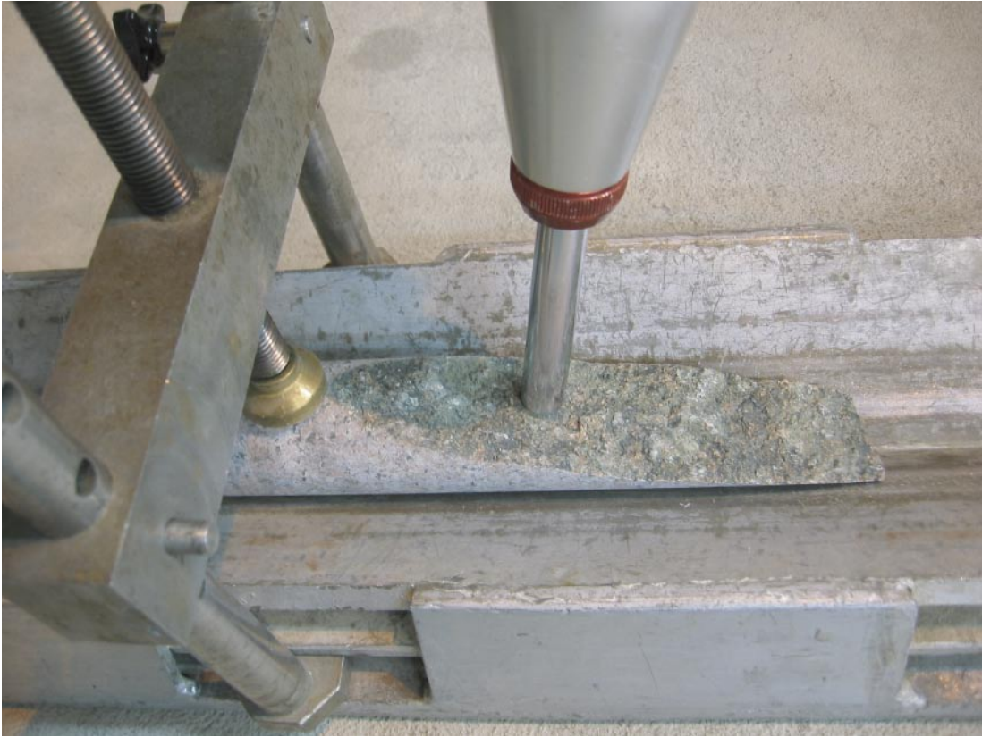
Figure 3-2. Clamp for the Schmidt hammer tests.
