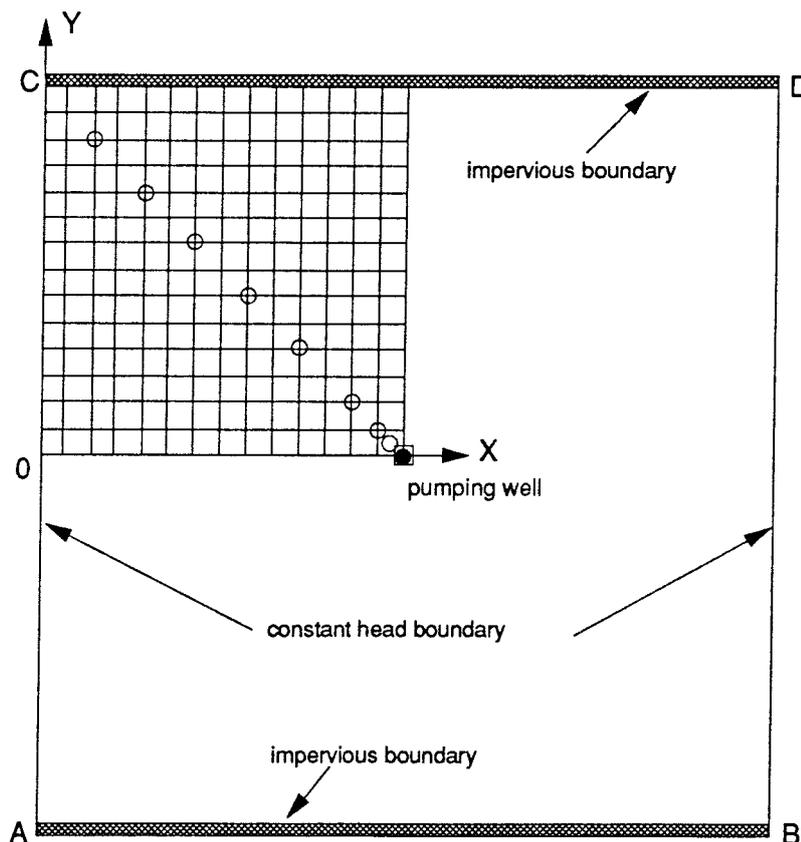
Figure A.6: Aquifer configuration and finite element discretization.
