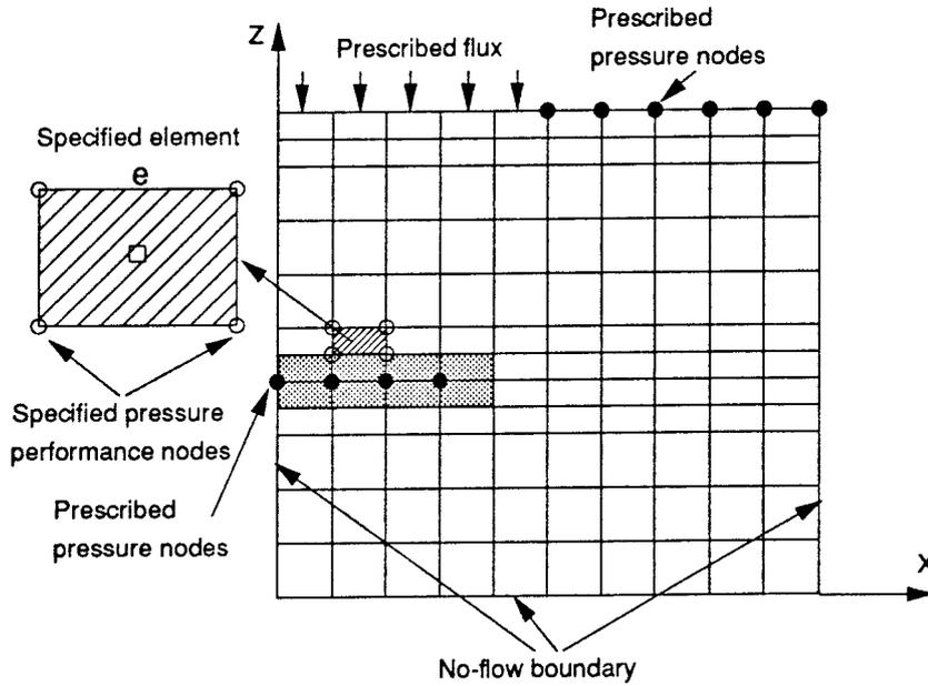
Figure 3: The element mesh of the flow domain
