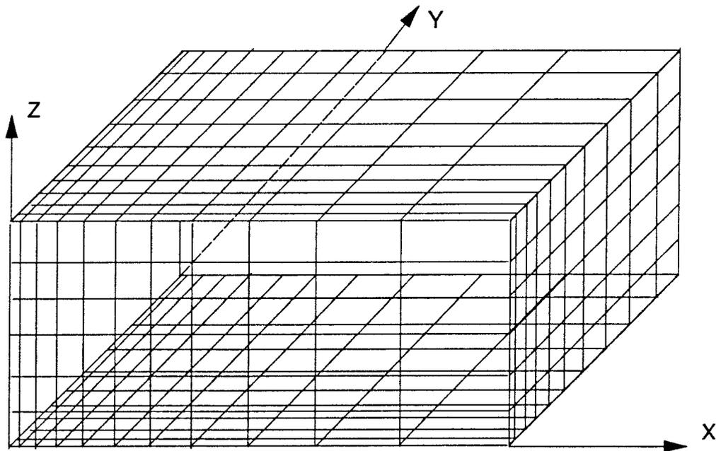
Figure A.4: Sample of 3-D unequal element mesh
