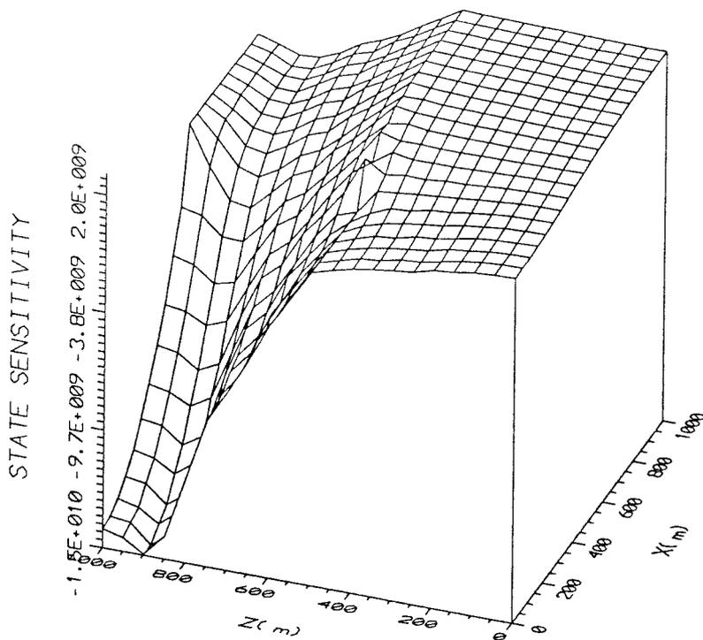
Figure 9: Perspective plot of state sensitivity for perturbing the second layer
