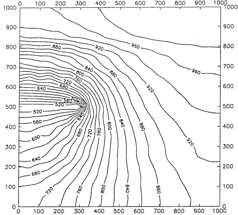
Figure 4: Contour map of the piezometric heads
