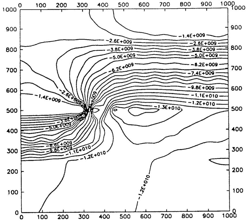
Figure 10: Contour map of state sensitivity for perturbing the third layer
