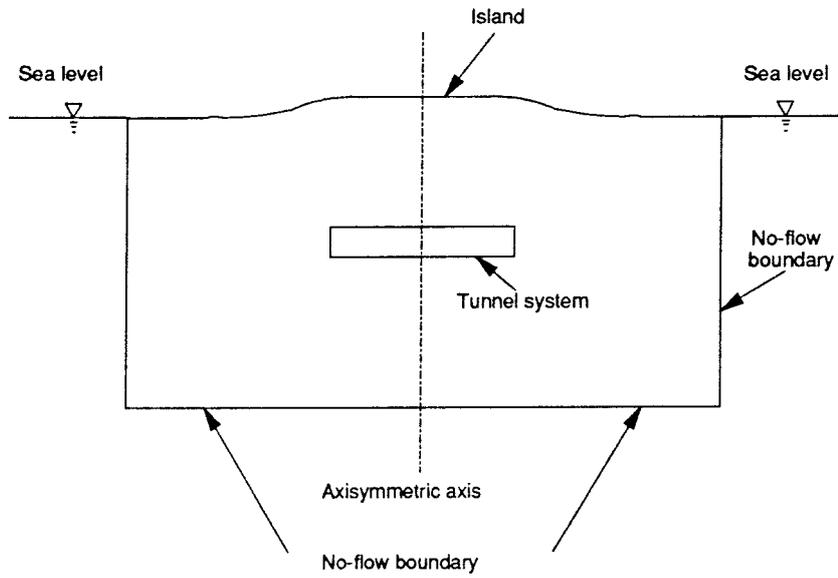
Figure 1: Schematic illustration of the flow domain
