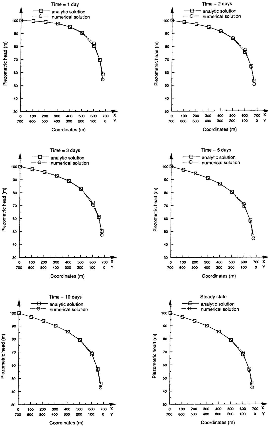
Figure A.7: Comparison of solutions of piezometric heads at transient state
