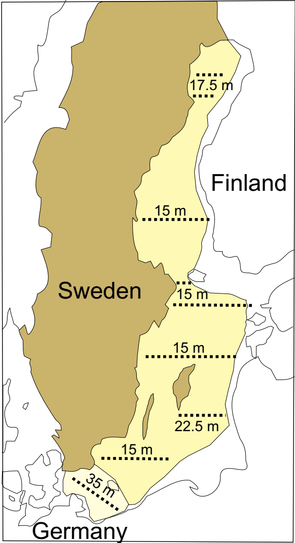
Figure 3-4. Estimation of sediment thickness within the Baltic basin along 8 profiles based on published data and estimates from geophysical data from the Institution of Geology and Geochemistry at the University of Stockholm. The positions of the profiles are shown by dotted lines and the numbers show the estimated average thickness of the deposits.
