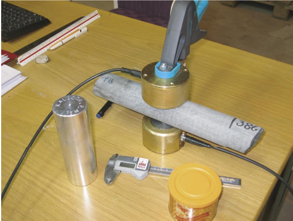
Figure G-2. Detail of NGI's apparatus for measuring acoustic P-wave travel time transverse borehole core. The aluminium cylinder for calibration of the device is on the left.
