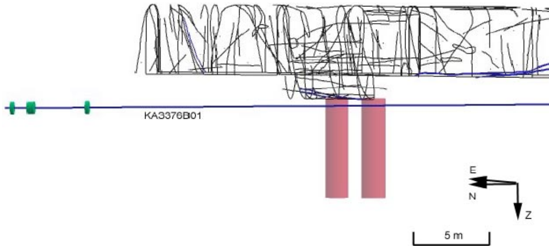
Figure 4-9. Localisation of samples collected for testing of fracture properties. The red cylinders represent the planned large holes.
