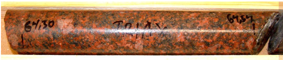
Figure 4-7. Picture of a oxidised sample of Äspö diorite.
