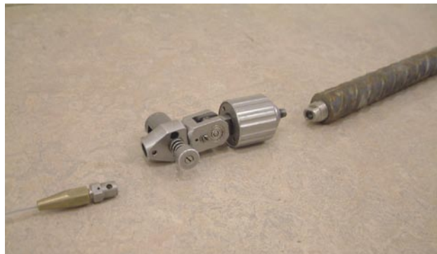
Figure 5-2. The approximate location of the seven pins in the pilot tunnel including example of three measured distances (left). Photograph of pin including screw tap and wire tap (right).
