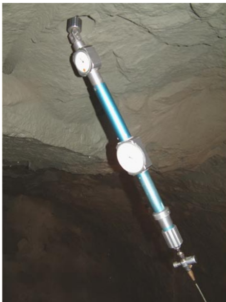
Figure 5-3. Photograph of Kern disotmeter attached at pin # 7 in the roof, note the countersink (left). The pins were installed approximately 0.3 to 0.5 m behind the face (right).
