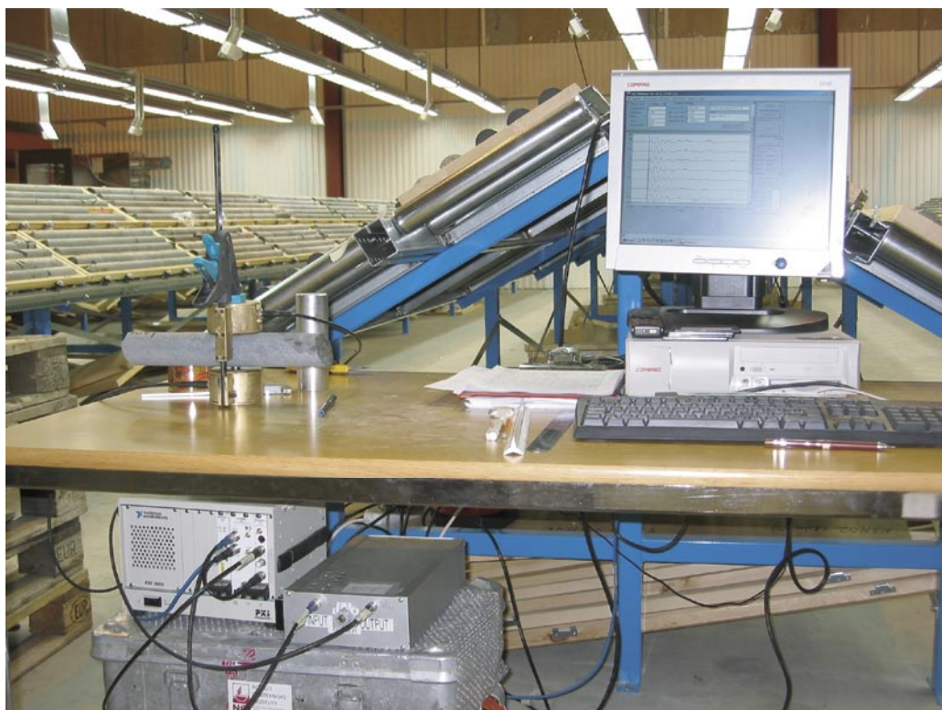
Figure G-1. NGI's equipment set up for measuring acoustic P-wave travel time transverse borehole core
