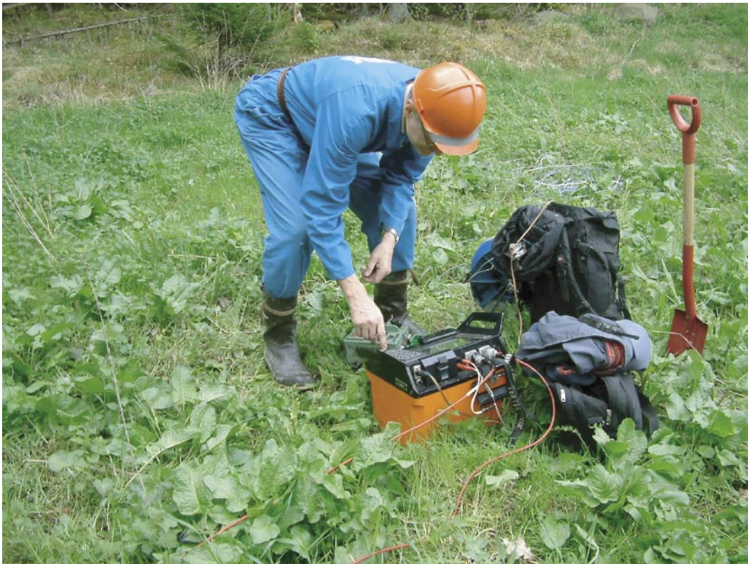
Figure 3-1. The recording instrument, ABEM Terraloc MK6.
