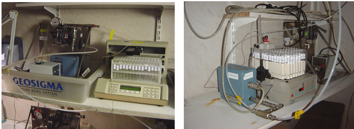
Figure 3-1. Tracer injection- (left) and sampling (right) equipment.
