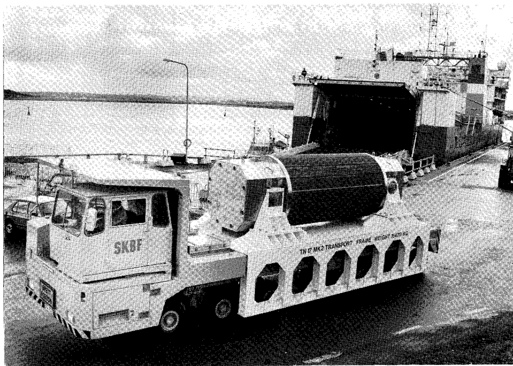
Figure 4-2. Transport vehicle with transport cask for spent nuclear fuel and M/S Sigyn in the background.
