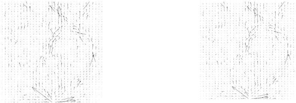
Figure 3-26. Velocities for relationships based on separation assumption (left) and mix assumption (right) at t=3.5 s.
