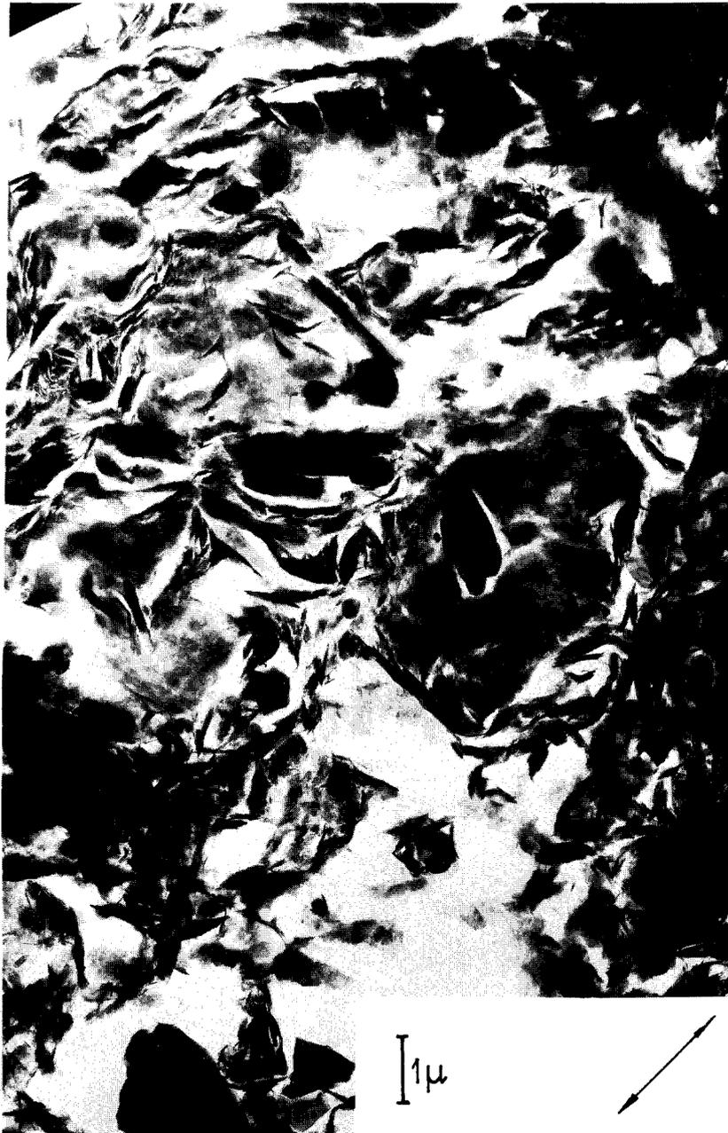
Fig 21. TEM micrograph of ultramicrotomed Silurian clay from Gotland. The arrow indicates the statistically certified general particle orientation
