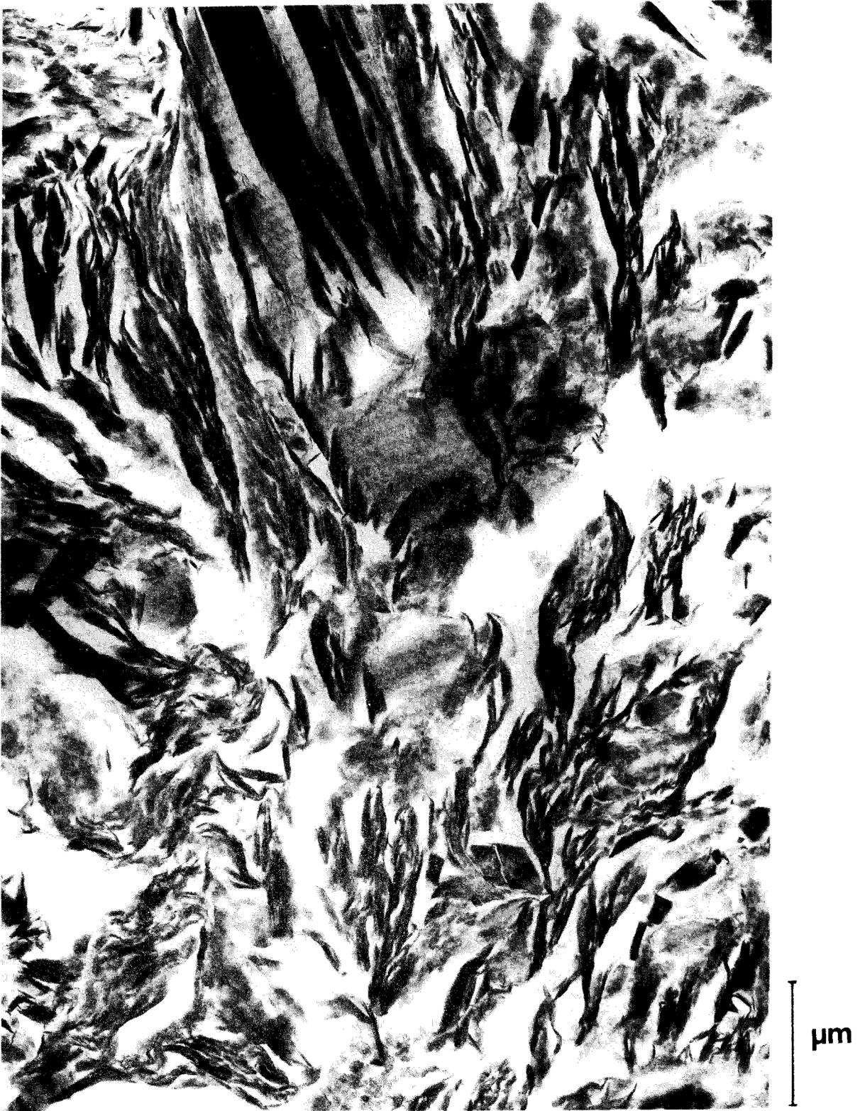
Fig 32. TEM micrograph of ultramicrotomed Boom clay showing strong particle orientation parallel to the bedding plane
