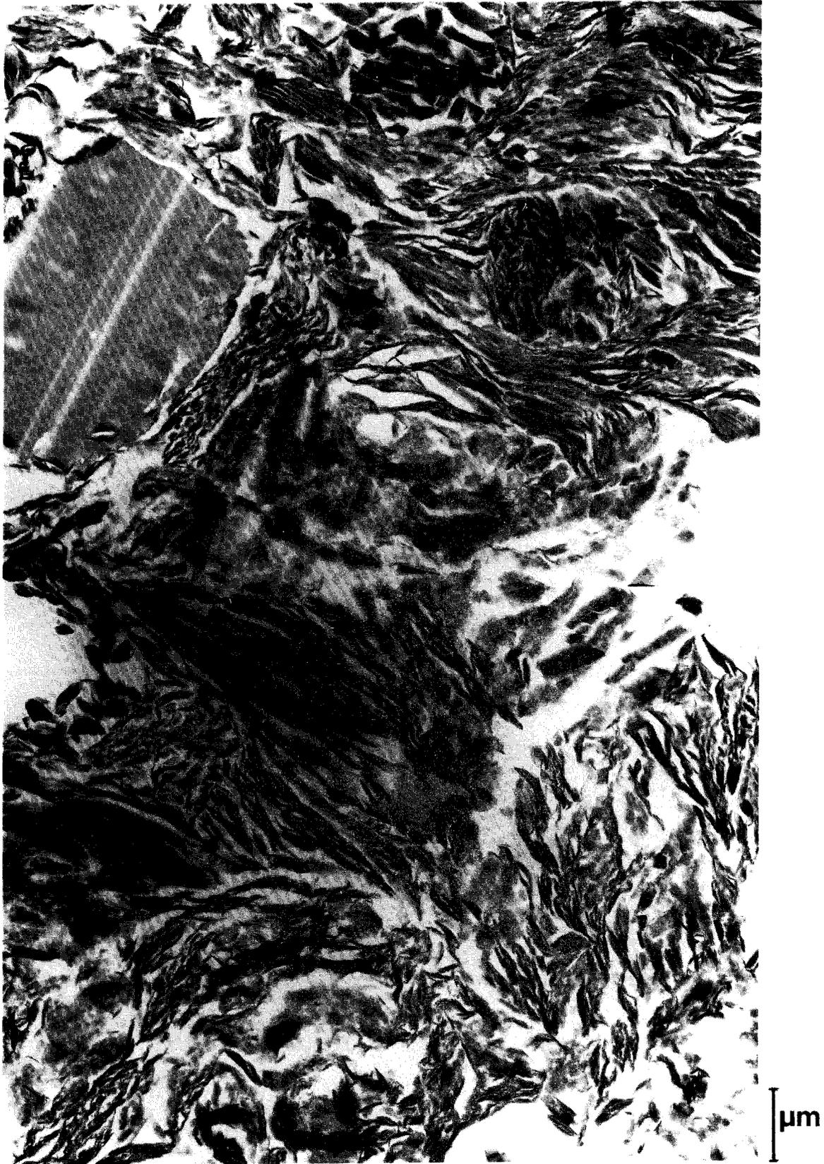
Fig 33. TEM micrograph of ultramicrotomed Boom clay showing strong domain formation due to shear stresses induced by the consolidation
