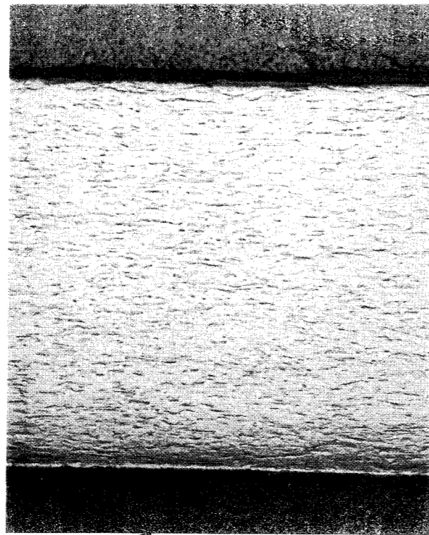
Clad. Etched for hydrides.
