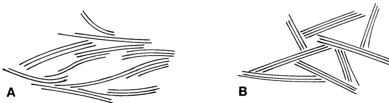
Fig 8. Microstructure of smectite clays at low bulk densities
